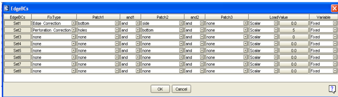
Fig. E.5 Boundary conditions for squeezed film damping for z-axis accelerometers
