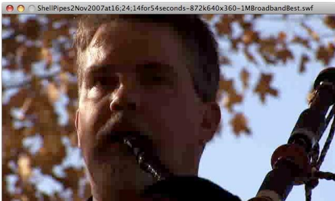
Figure 4.5 VP6 CBR encoded frame show significant blockiness [36][39]
