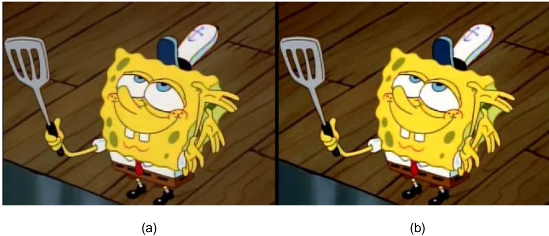
Figure 3.1 Saturation of colors (a) VP6 – true to original (b) Flash MX - oversaturation of colors [25]
