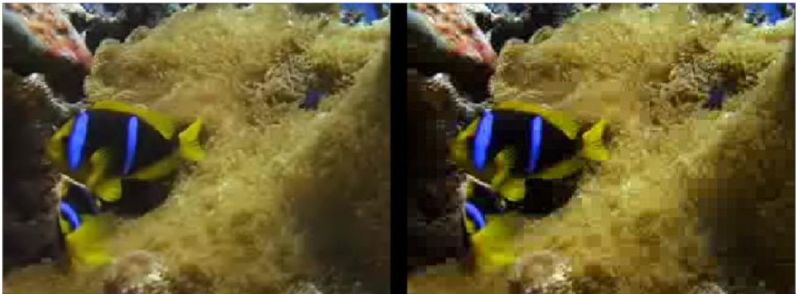
Figure 3.2 (a) VP6 – Better quality picture (b) Flash MX - Blockiness of the subject and background [25]
