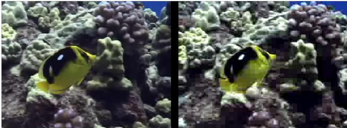
Figure 3.2 (a) VP6 – Better quality picture (b) Flash MX - Blockiness of the subject and background [25]
