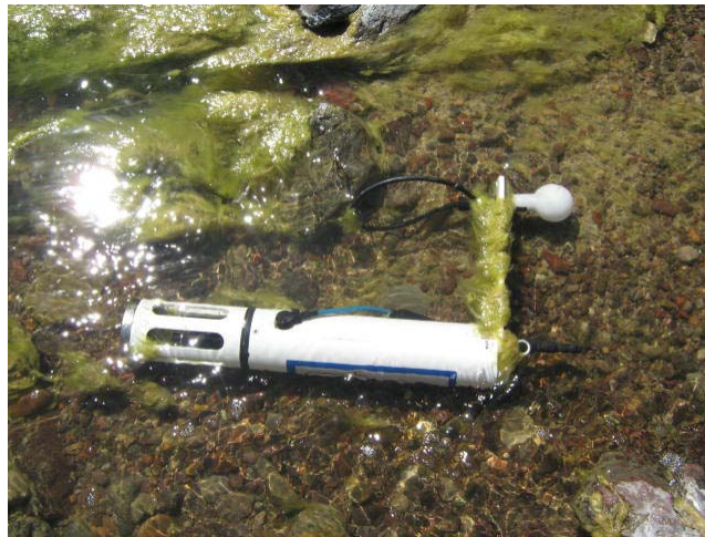
Figure 2.9 Image of the HydroLab Datasonde deployed in March 2007.
