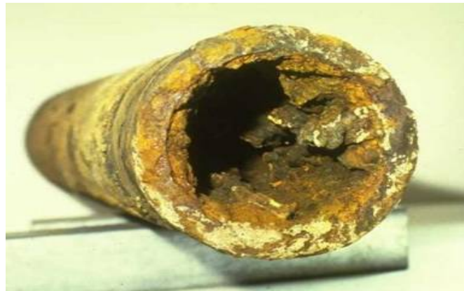
Figure 1.1 - Effects of Tuberculation, Age and Corrosion on Water Pipes (Source: 3M Water Infrastructure)
