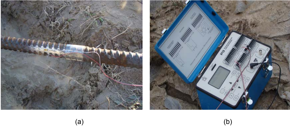
Figure 6.12. Strain Gauge Instrumentation: (a) Gauge Attached, and (b) Data Receiver
