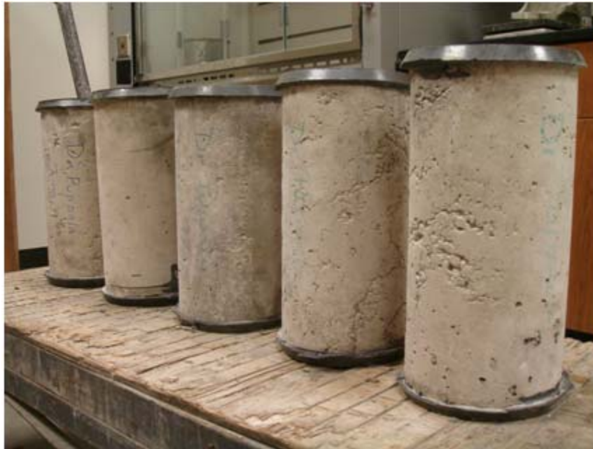
Figure 5.17. Concrete Cylinder Specimens with Capping Compound
