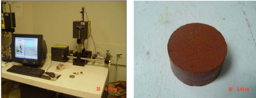
Figure 3.4. The Direct Shear Test Setup and Compacted Silty Sand Used in the Test
