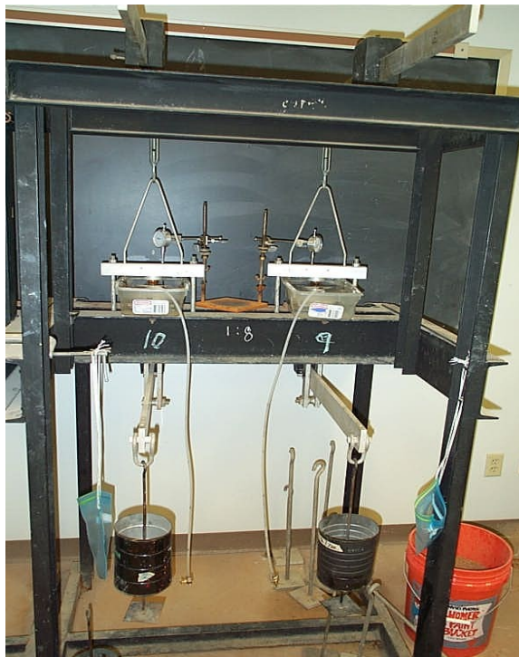
Figure 3.6. One-Dimensional (1-D) Swell Pressure Test Setup
