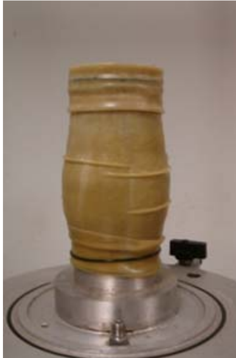
Figure 3.5. Typical Failed Triaxial Specimen
