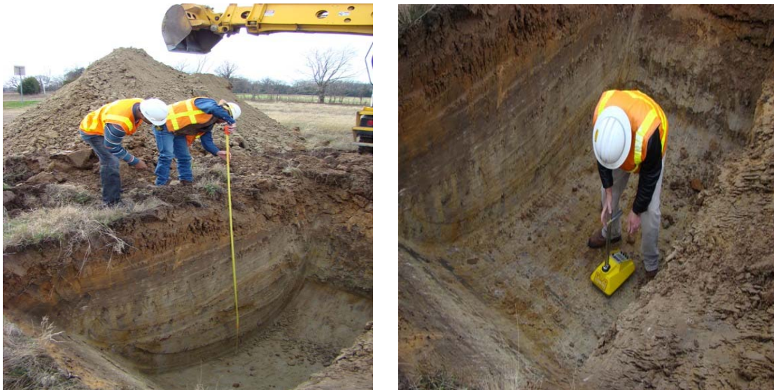
Figure 3.2. Soil Sampling and Field Density Measurement by Using a Nuclear Density Gauge
