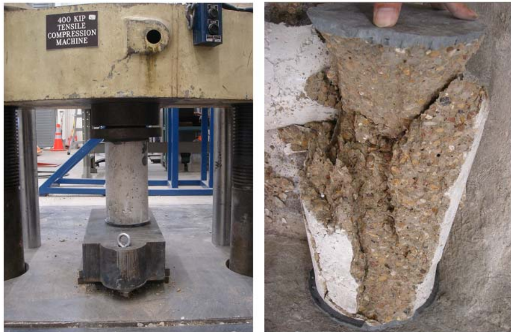
Figure 5.18. The 400 kip Tinius Olsen Tensile and Compression Machine used for Testing
