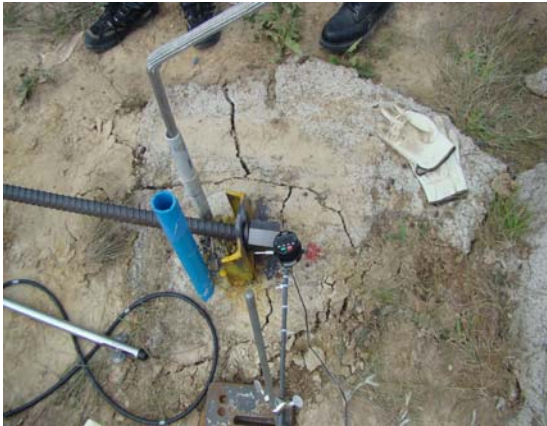
Figure E.9. Summer Condition Test Shaft Concrete Failures
