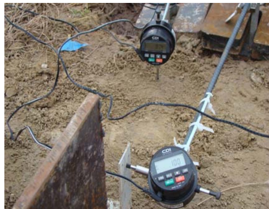
Figure E.7. Measuring Lateral and Vertical Displacement (Summer and Winter Conditions)
