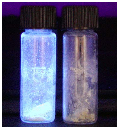
Figure 5.12 Xerogels 76 obtained upon bubbling \text{CO}_2 to benzene (left) and benzene-nitrobenzene, 95:5 (right) solutions of 73 .
