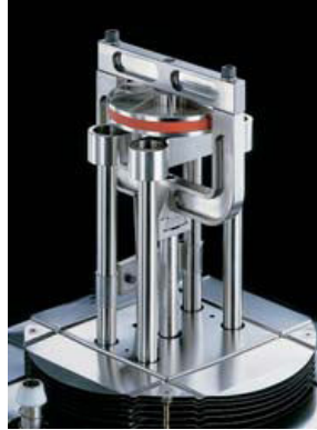
Figure 2 Compression Clamp- fixed flat surface and an oscillating plate applies force. 1
