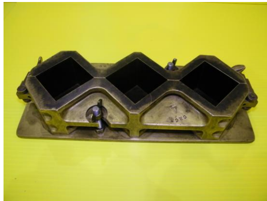
Figure 4.10 Brass Mortar Cube Mold
