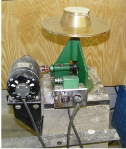
Figure 4.8 Flow Table with Mold
