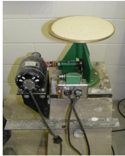
Figure 4.9 Flow Table after 25 Drops
