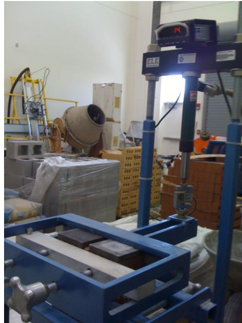
Figure 4.27 Clay Brick Bond Wrench Machine
