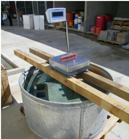
Figure 4.13 Immersed Weight Measurement
