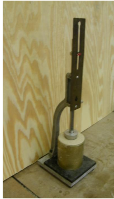
Figure 4.20 Cone Penetration after Release
