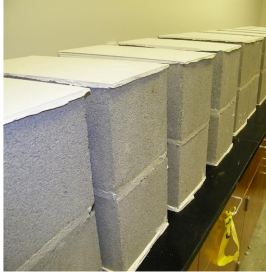
Figure 4.25 Capped Compression Prisms
