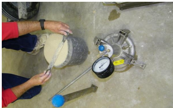
Figure 4.21 Air Content by Pressuremeter
