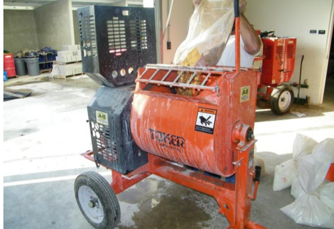
Figure 4.17 Professional Mason Operating Mechanical Mixer
