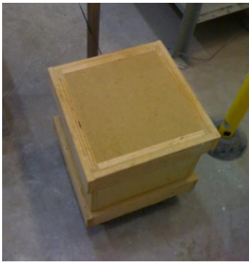
Figure 4.15 Plywood Box for Sand
