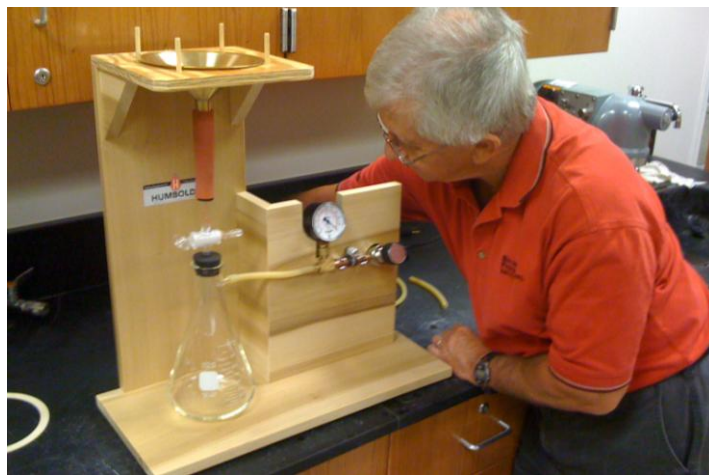
Figure 4.12 Suction Apparatus for the Water-Retention Test
