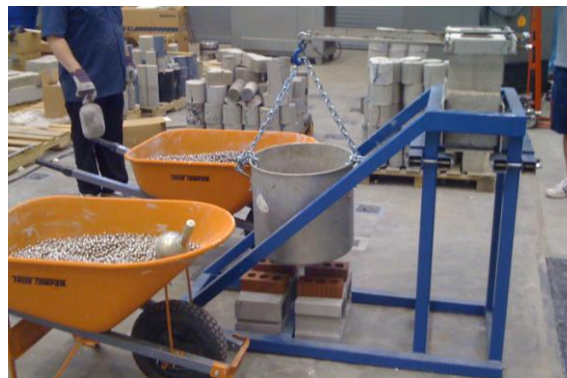
Figure 4.28 Concrete Bond Wrench Testing
