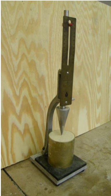
Figure 4.19 Cone at Initial Setting
