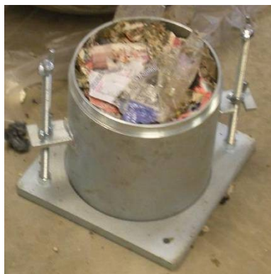
Figure 3.8 Fully Compacted MSW in Compaction Mold
