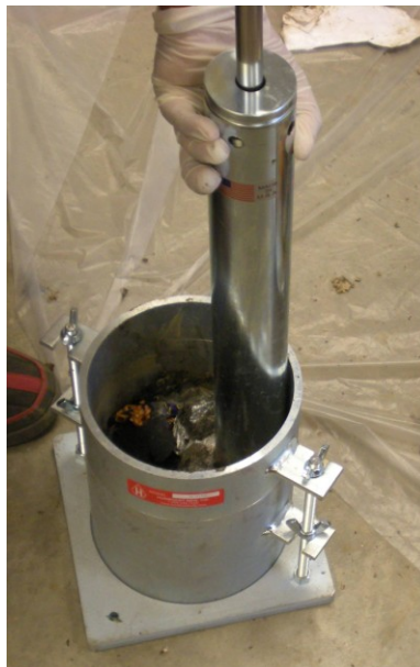
Figure 3.7 Sample being Compacted at First Layer
