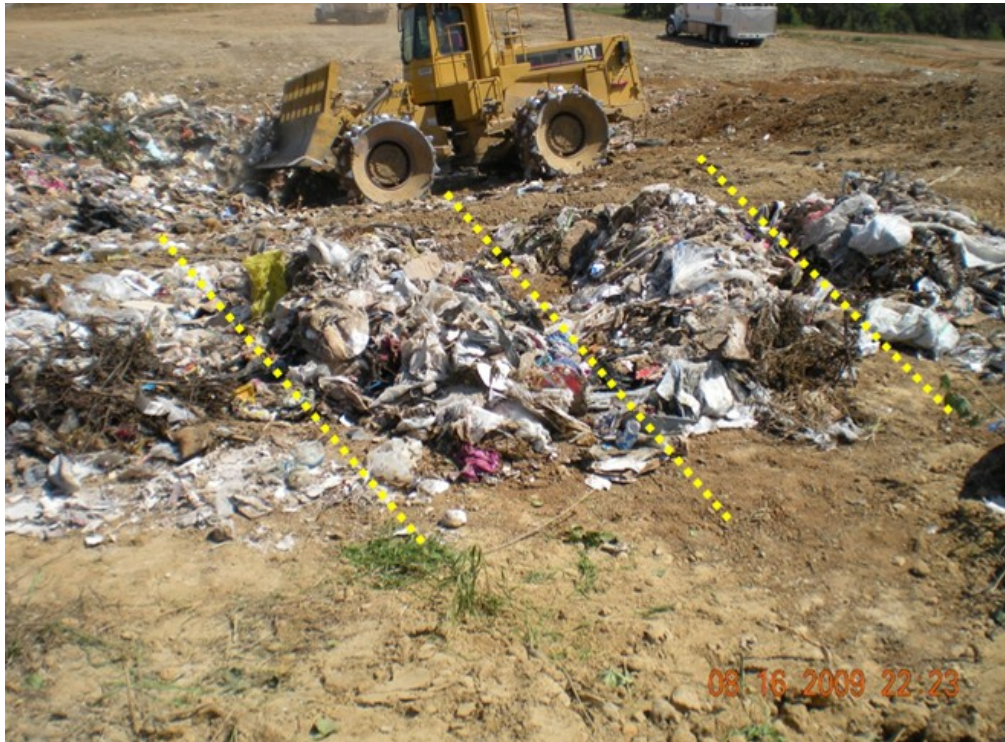
Figure 3.1 Quartering Solid Waste with a Backhoe
