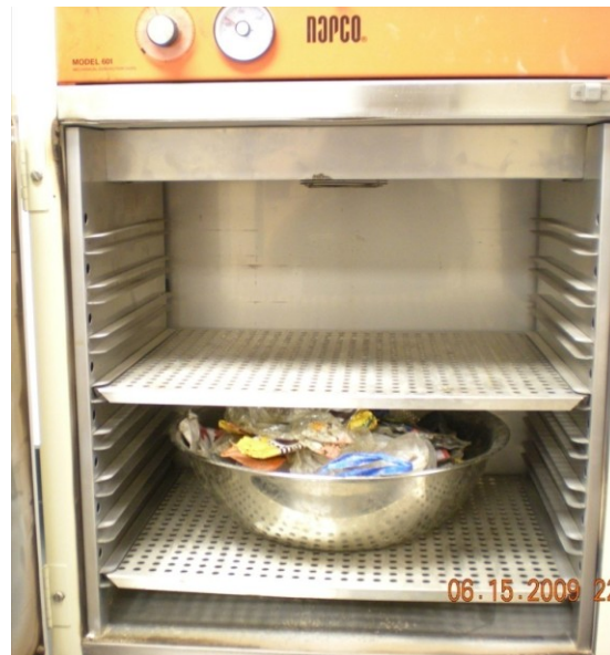
Figure 3.6 Sample Placed in Oven for Determination of Moisture Content
