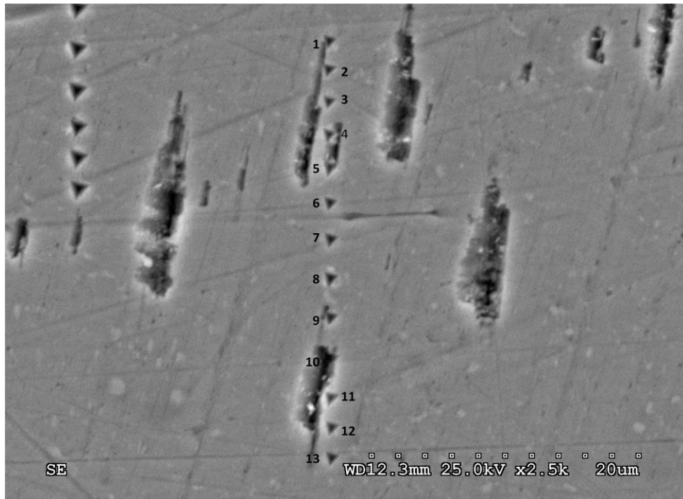
Figure 6.3 SEM image of Group 3 indents on FA cooled SAC405 matrix
