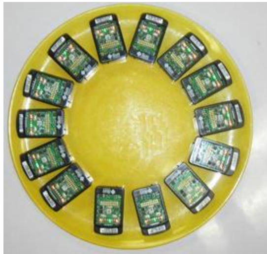
Figure B1 – SunSpot minicomputers equipped with temperature, light, and acceleration sensors.
