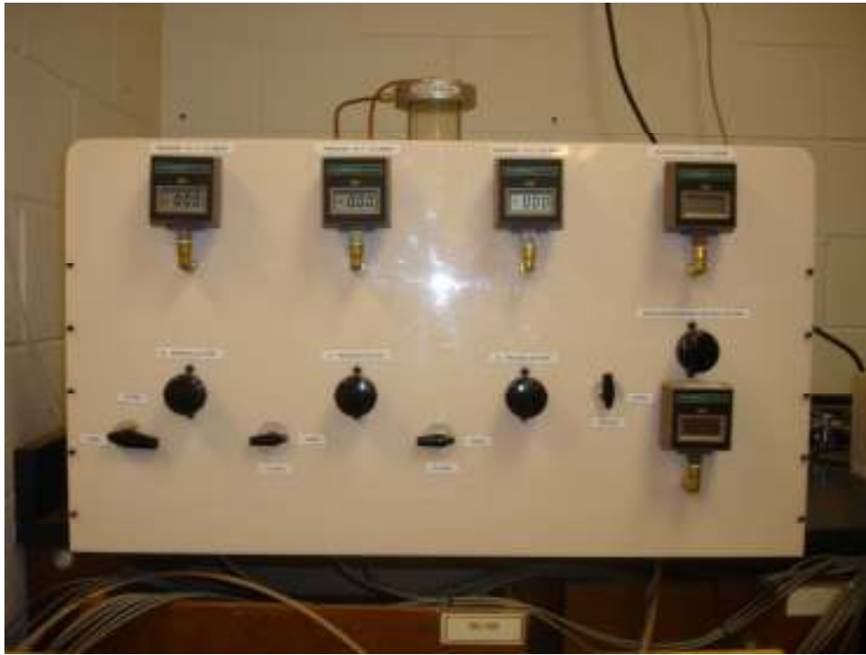
Figure 3.5 Photograph of Stress Control System
