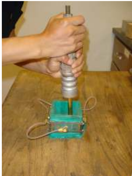
Figure 4.3 Photograph of Kneading Compaction for Specimen Preparation
