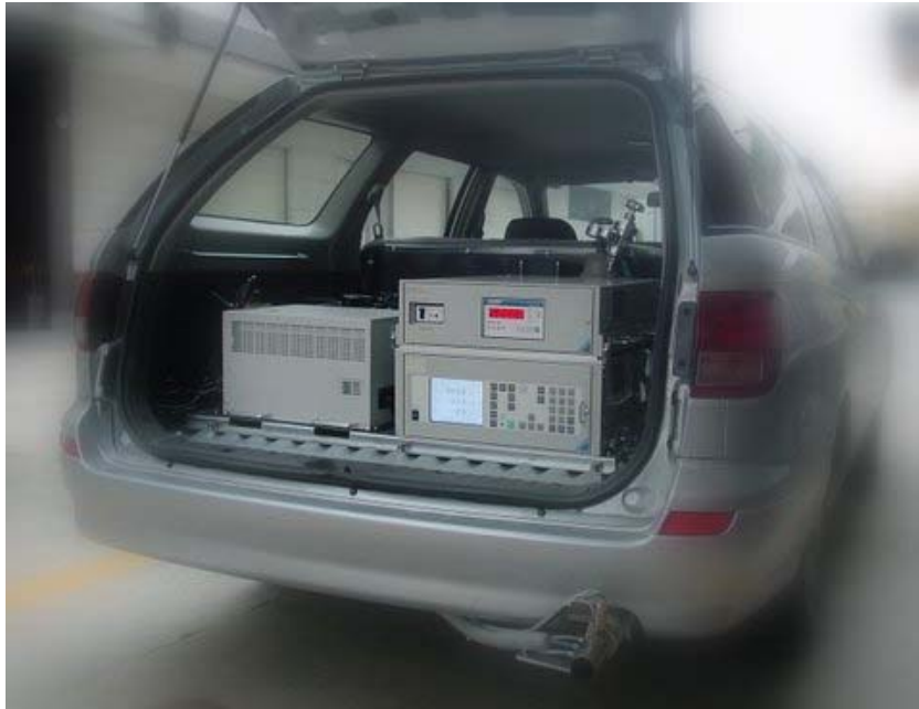
Fig 2.3 On-Board measurement System
