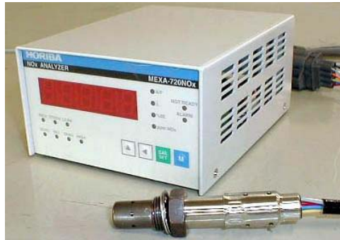
Figure 3.7 MEXA-720 unit and NO x sensor
