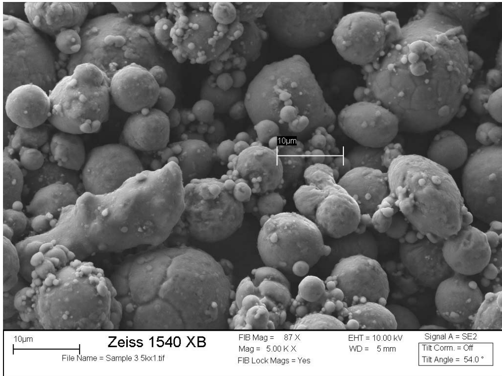
Figure A.9 SEM image of ABM coatings (8-12 µm)
