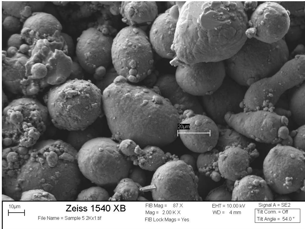
Figure A.11 SEM image of ABM coatings (17-30 µm)
