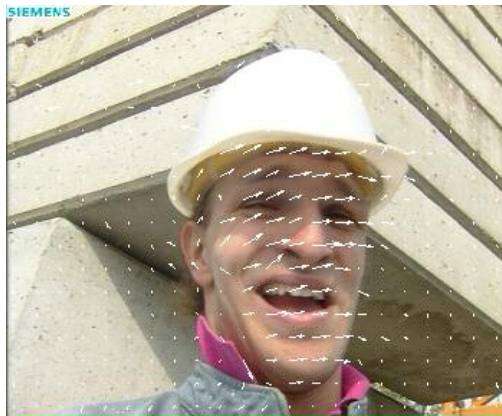
Fig. 5.18 P frame of 1Mbps clip foreman in MPEG-2 transcoded stream with motion vectors marked
