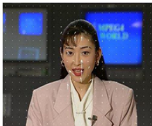
Fig 5.21 P frame of 1 Mbps clip Akiyo in MPEG-2 transcoded stream with motion vectors marked
