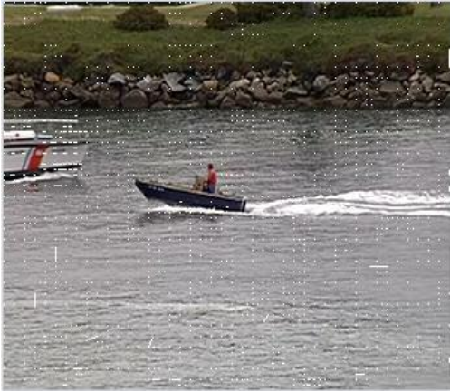
Fig 5.23 P frame of 1Mbps clip coastguard in H.264 stream with motion vectors marked.
