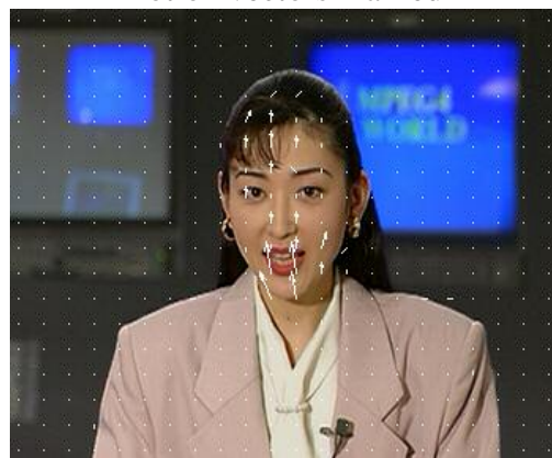
Fig. 5.22 P frame of 1Mbps clip Akiyo in MPEG-2 encoded stream with motion vectors marked.
