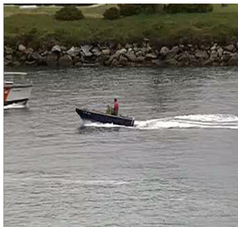
Fig 4.16 Subjective quality of an I frame of the clip Coastguard in a 3.4 Mbps transcoded MPEG-2 stream.
