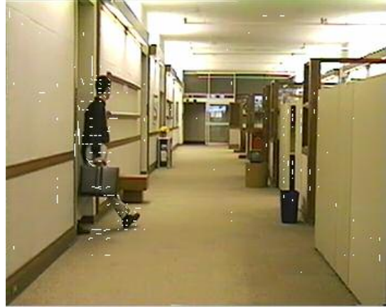
Fig.5.26 P frame of 1Mbps clip hall monitor in H.264 stream with motion vectors marked.
