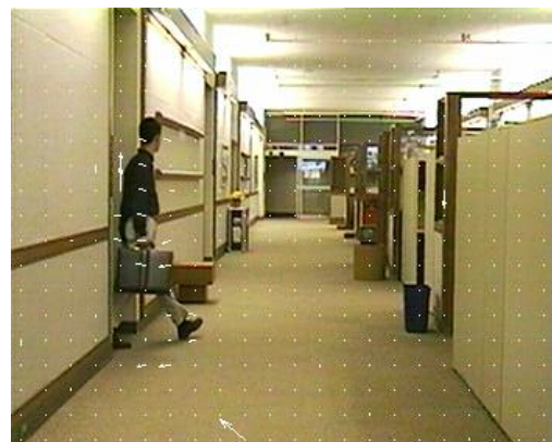
Fig.5.28 P frame of 1Mbps clip hall monitor in MPEG-2 encoded stream with motion vectors marked.
