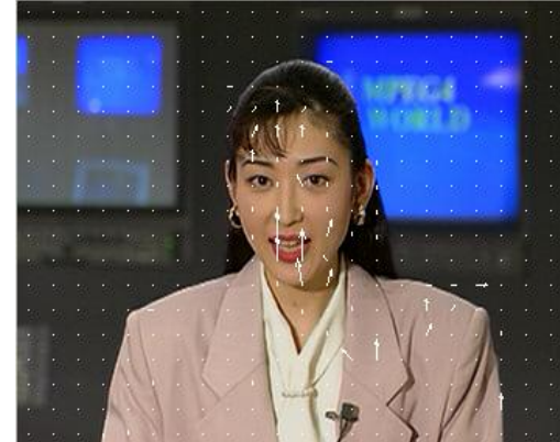
Fig 5.33 P frame of 1 Mbps clip Akiyo in MPEG-2 transcoded stream with average motion vectors marked
