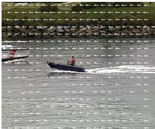
Fig.5.25 P frame of 1Mbps clip coastguard in MPEG-2 encoded stream with motion vectors marked.
