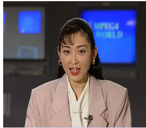
Fig 5.20 P frame of 1Mbps clip Akiyo in H.264 stream with MVs marked.
