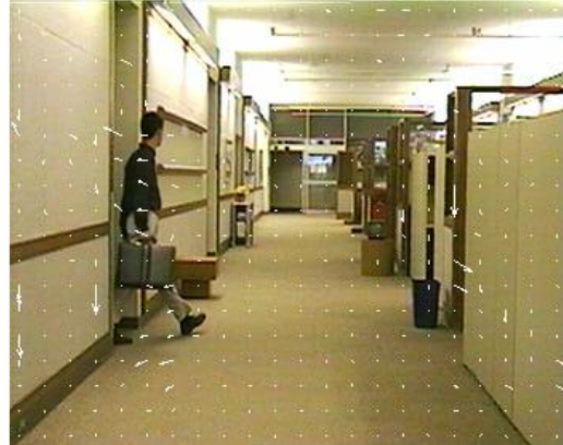
Fig.5.27 P frame of 1Mbps clip hall monitor in MPEG-2 transcoded stream with motion vectors marked.
