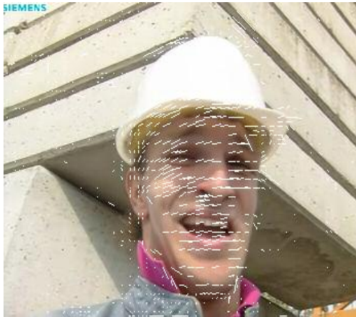
Fig. 5.17 P frame of 1Mbps clip foreman in H.264 stream with motion vectors marked
