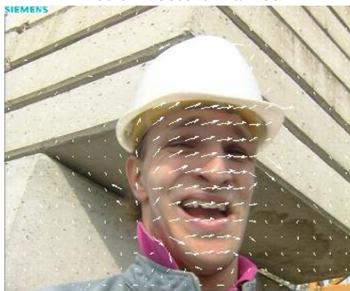
Fig. 5.19 P frame of 1Mbps clip foreman in MPEG-2 encoded stream with motion vectors marked
