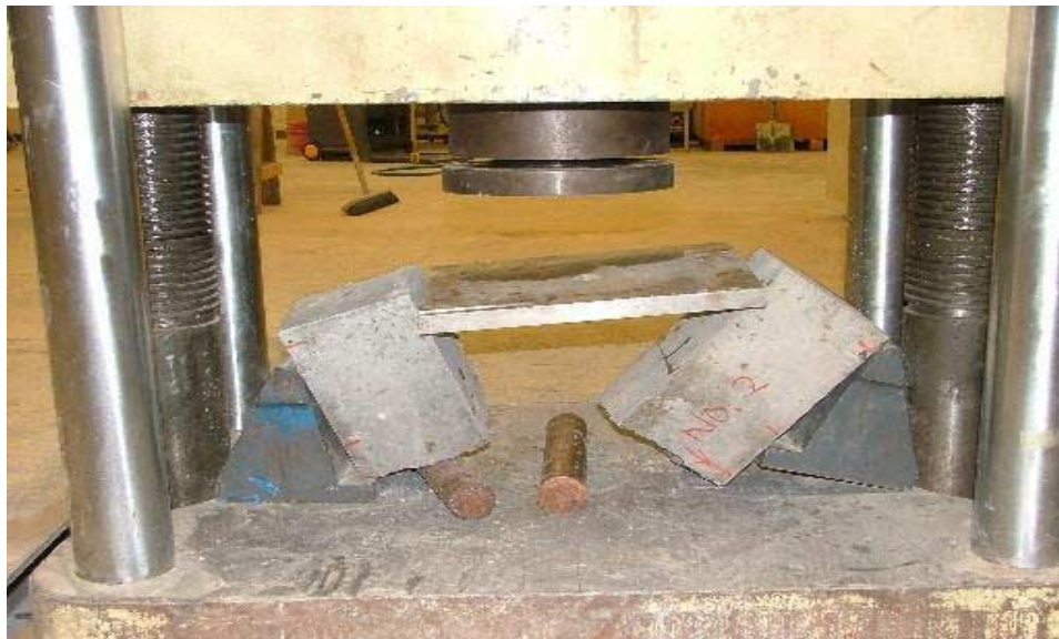
Figure 2.11 Failure of Concrete Specimen
