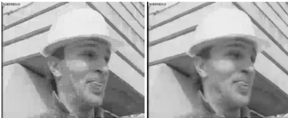
Figure 1.16: Performance of the deblocking filter for highly compressed pictures. Left: without deblocking filter, right: with deblocking filter. [16]
