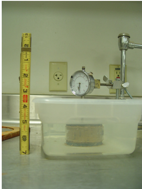
Figure 3.5 Free swell setup on treated soil specimen
