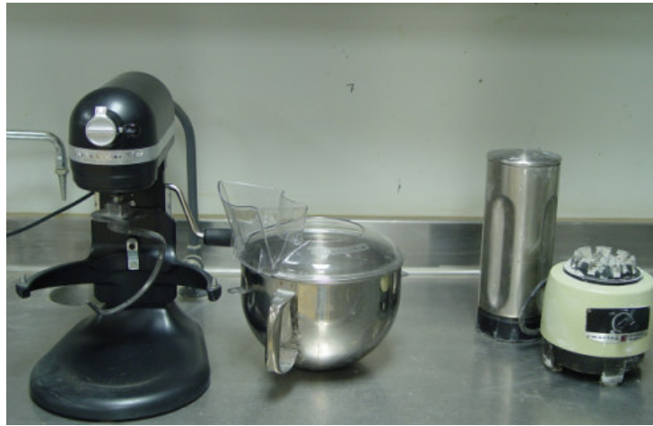
Figure 3.2 Domestic mixer to simulate mixing procedure and commercial blender for slurry preparation (Bhadriraju 2005)
