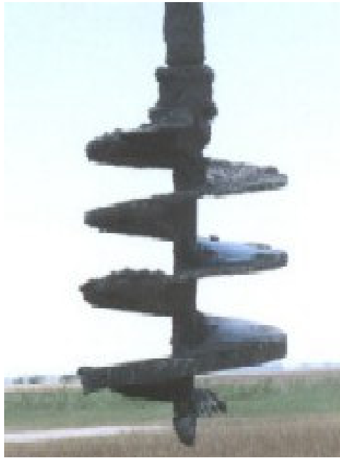
Figure 2.2 Example of single-shafted site auger ( http://www.dot.state.fl.us/ )
