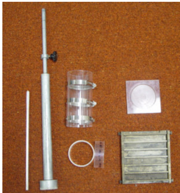
Figure 3.3 Details of compaction rammer, poking rod, free swell mold, UCS mold, base plate and linear shrinkage mold
