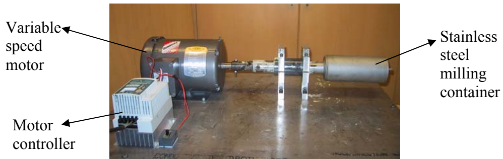
Figure 4.2 The ball milling set-up for milling of NaCl powders
