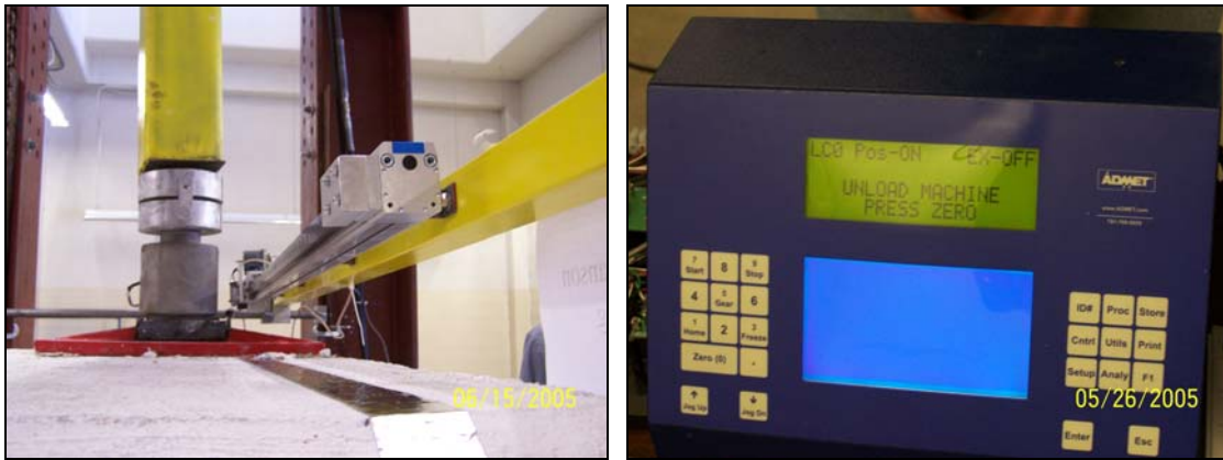
Figure 2.14: Load Cell, Self-Leveler and Admet® Controller
