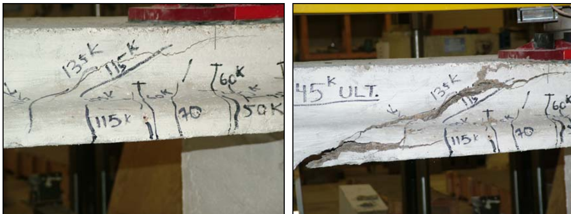
Figure 3.14: Test Three Failure
