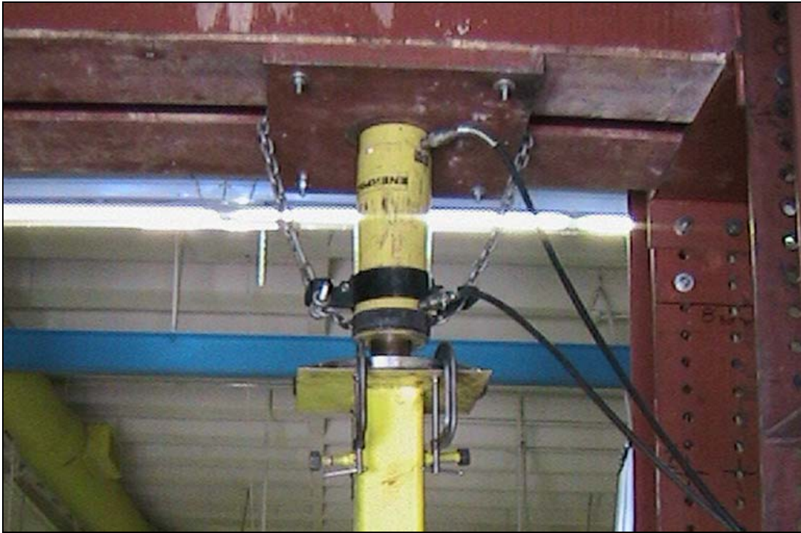
Figure 2.13: Inverted Hydraulic Jack and Transfer Column
