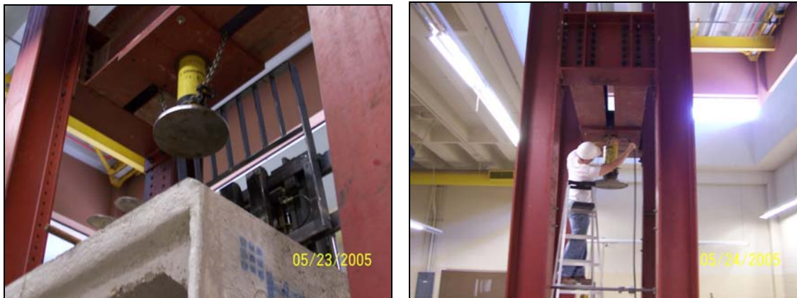
Figure 2.3: Transfer Girder with Hydraulic Jack
