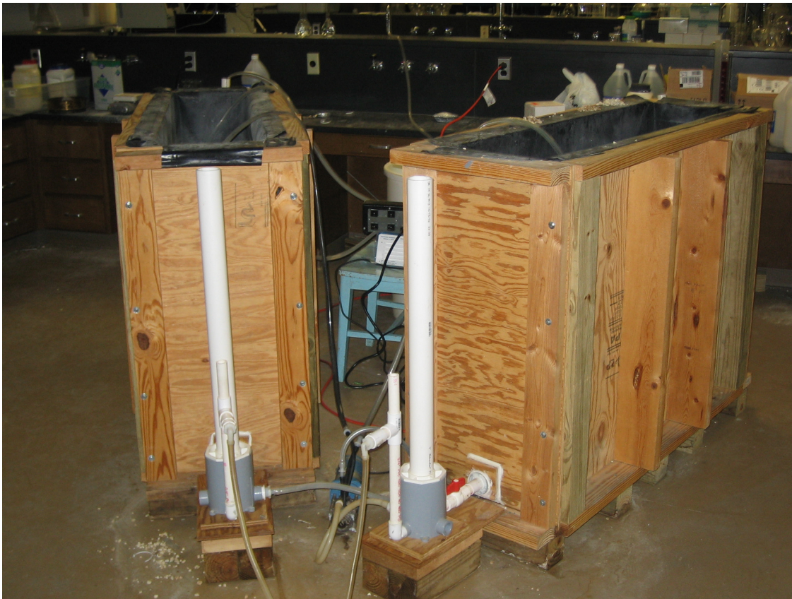
Figure 3.1 Two pilot scale biofilters for laboratory experiments
