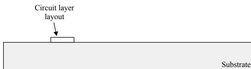
Figure 5.1 Circuit layer is first fabricated on the substrate.
