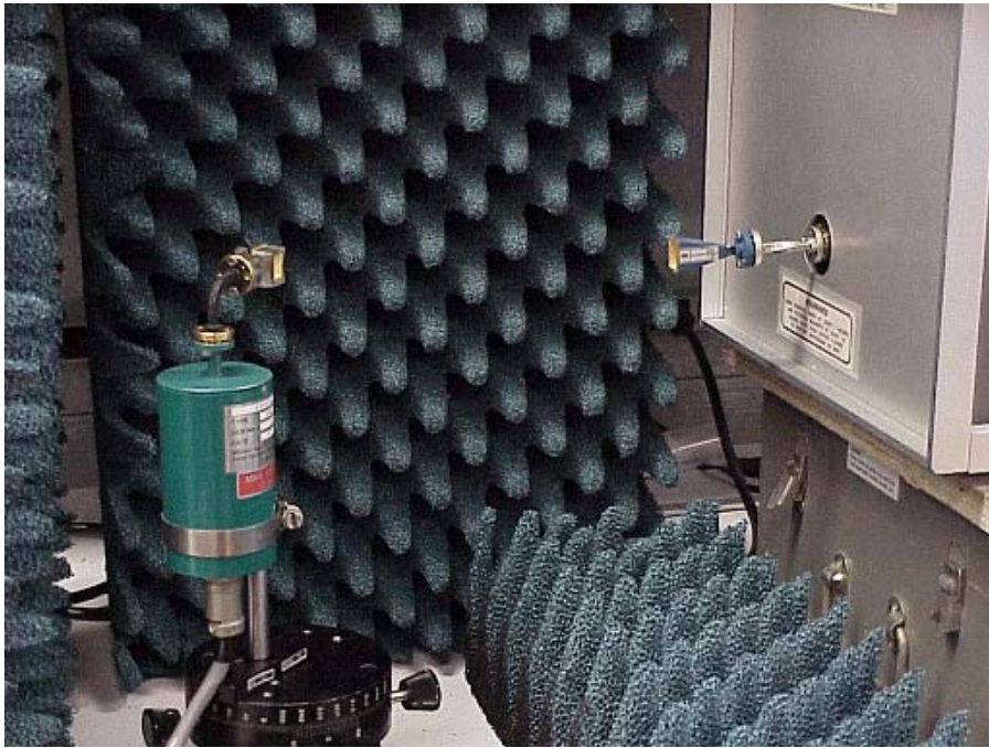
Figure 2.43 The micro hot embossed horn antenna measurement set up.
