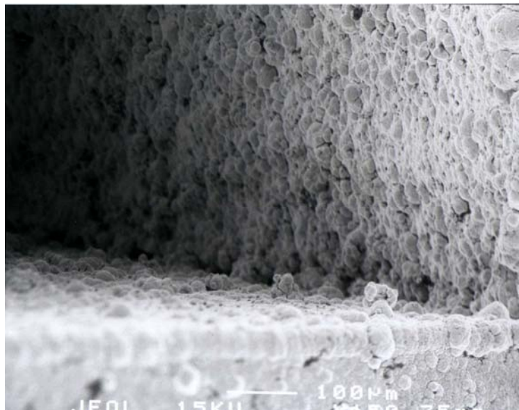
Figure 2.7 SEM photo of a close view of the lower right corner of the rectangular waveguide.
