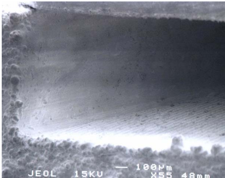
Figure 2.6 SEM photo of the lower left corner of the rectangular waveguide.
