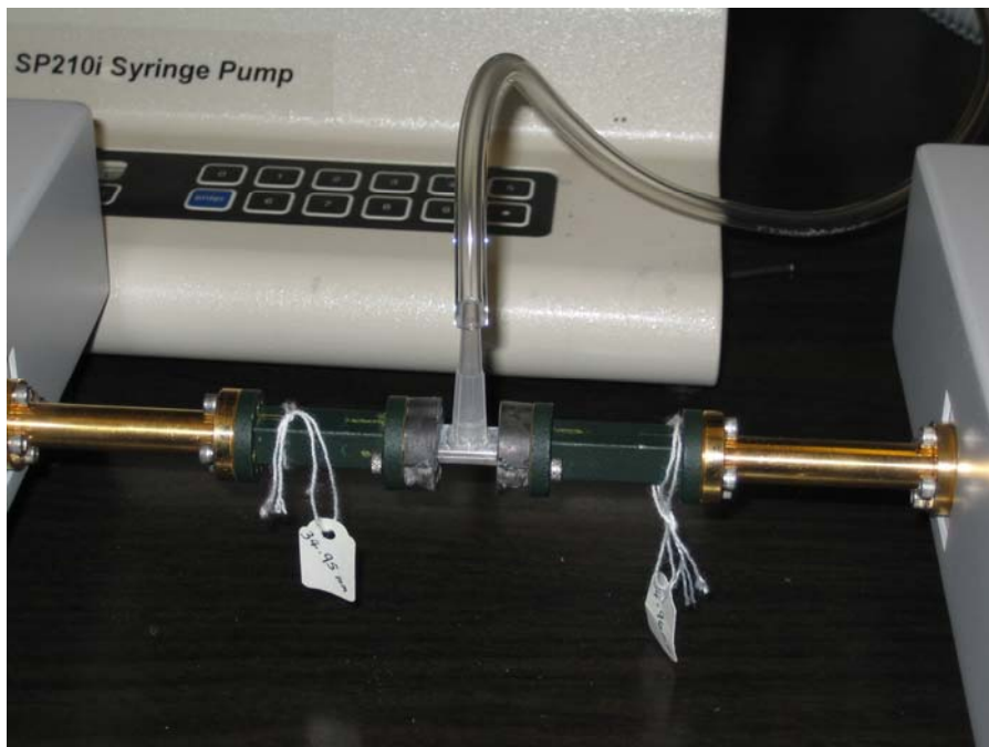
Figure 4.9 Measurement set up of the prototype tunable filter [4.1].
