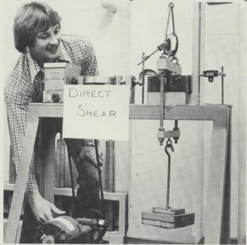
Above: Jim Oberg is running a direct shear soil test.
