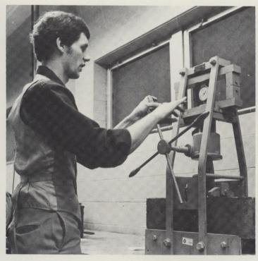
Kerry Kennedy runs flexual tension test on concrete beams.
