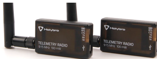
Figure 4.6. Holybro SiK 915MHz telemetry radio.
