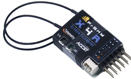
Figure 4.5. FrSky X4R-SB RC Receiver.
