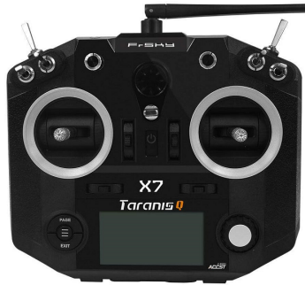
Figure 4.12. FrSky Taranis Q X7 RC transmitter.
