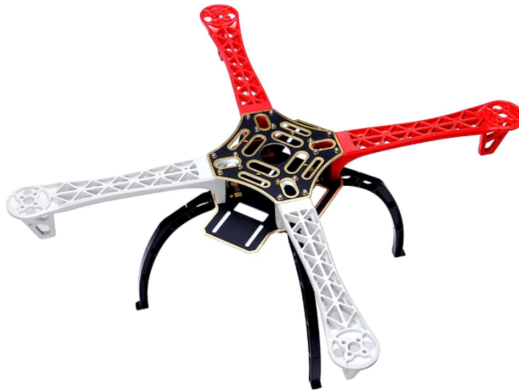
Figure 4.3. DJI F450 Airframe.
