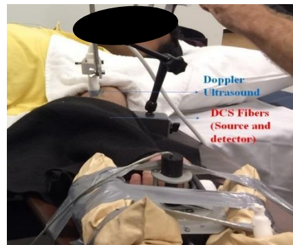
Figure 19(a): DCS Probe covered with a black cloth and Doppler ultrasound on the brachial artery together
