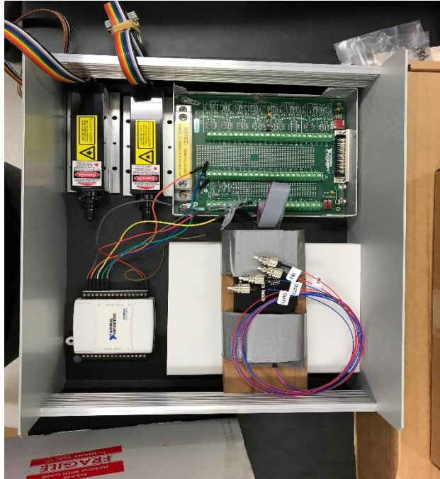
Figure 31(d): Photograph of the hardware enclosure for dual wavelength DCS system.
