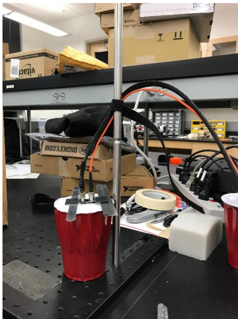
Figure 33(b): Photograph of probe placement during intralipid phantom test.
