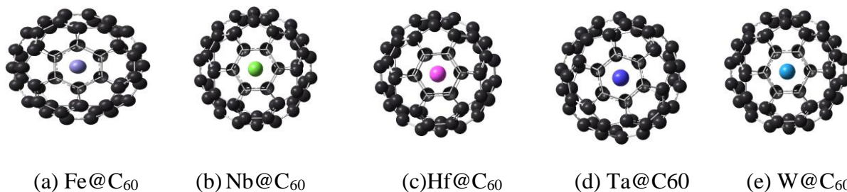
Figure 4.1.1: showed the relaxed structures of M@C 60 fullerene, where M= Fe at (a), Nb at (b), Hf at (c), Ta at (d), and W at (e).
