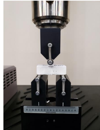
Figure 0.2: (a) Shear force and bending moment diagram, (b) experimental setup for 3-point bending test
