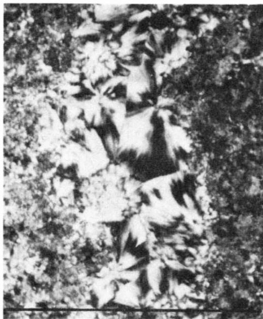
D. Chalcedonite cavity filling in dolomite, slide P-7-3, crossed nicols.
