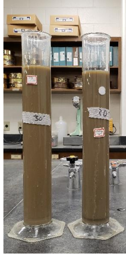
Figure 3-4: Particle size distribution testing using the hydrometer procedure
