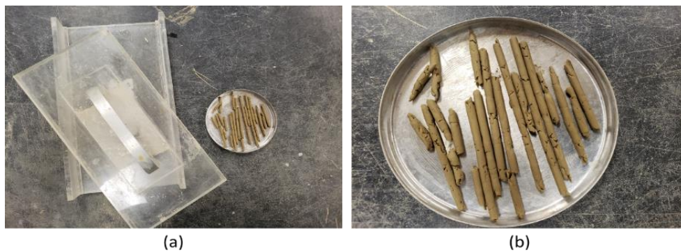
Figure 3-6: Rolling device and cracked and shattered threads of 3 mm plastic limit testing
