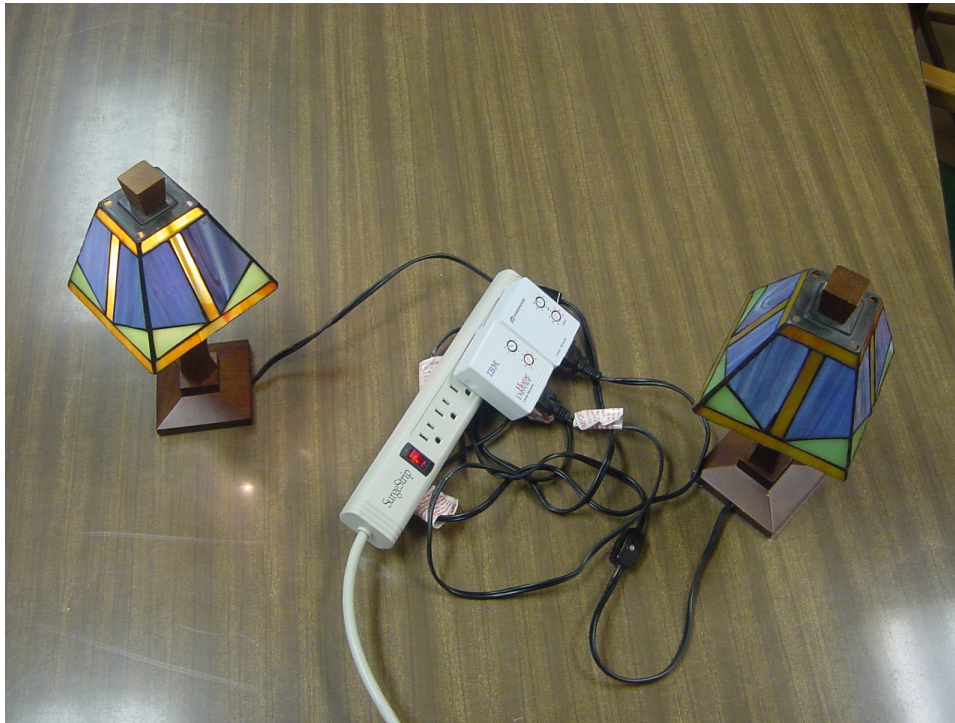
Figure A.4. X-10 lamp modules and connected lamps.
