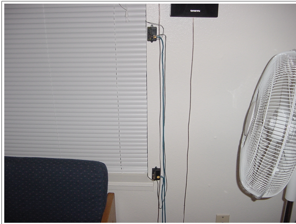
Figure C.6. ArgusMS Dongle sensors by the window near an X-10 controlled floor fan.
