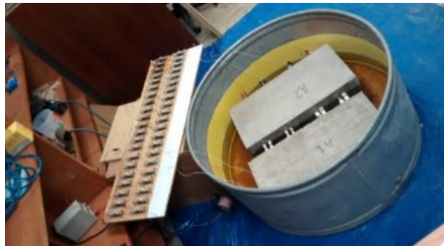
Figure 2- 12: Accelerated corrosion setup (Raju et al., 2018)
