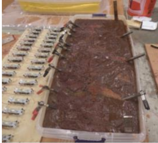
Figure 2- 14: Tank for accelerated corrosion (Hasan & Yazdani, 2015)
