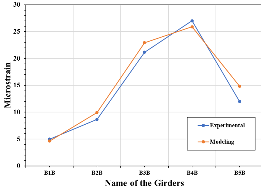
Figure 6- 44: Comparison of the strain data between the experiment and the ABAQUS model
