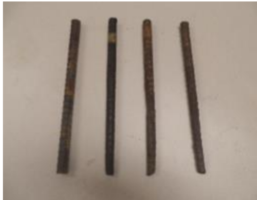
Figure 2- 15: Rebars with different degrees of corrosion (Hasan & Yazdani, 2015)
