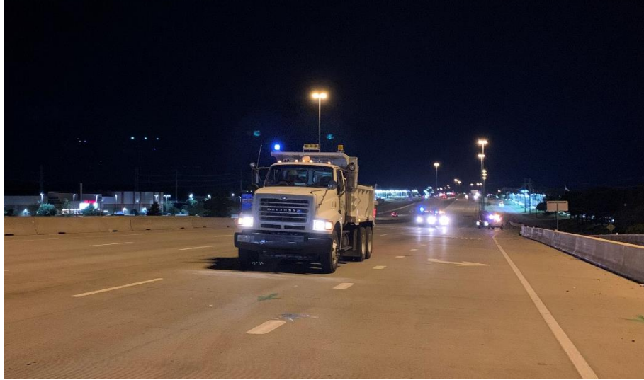
Figure 4- 24: Dump truck for vibration test during static load testing
