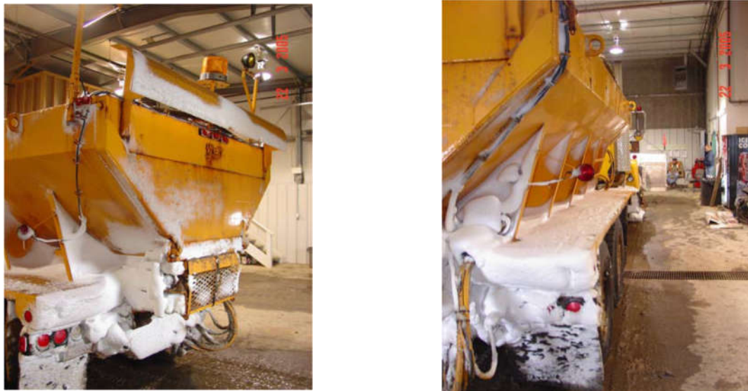
Figure 3-31 Wind deflector tests by Alberta Infrastructure and Transportation (Paulichuk, 2005) show extensive snow accumulation on the rear of a winter operations vehicle, despite having wind deflectors over taillights.
