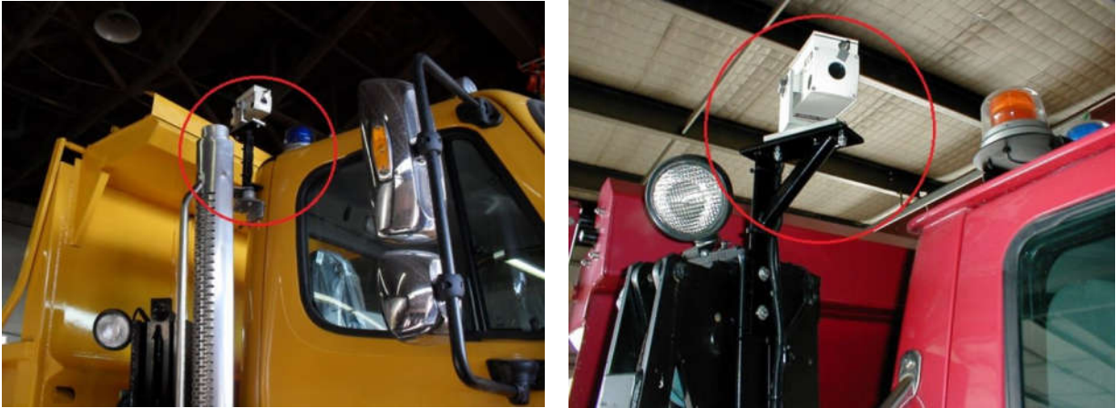
Figure 3-44 Two different winter operations vehicles with laser projection equipment installed on them (Laserline, 2018)
