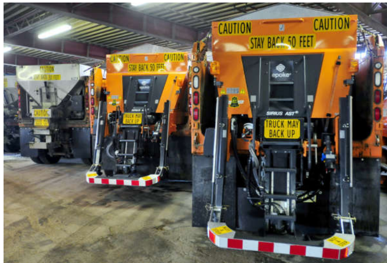
Figure 3-12 Winter operations vehicles in Saginaw County (Michigan) with message signs at the back (Saginaw News, 2012)
