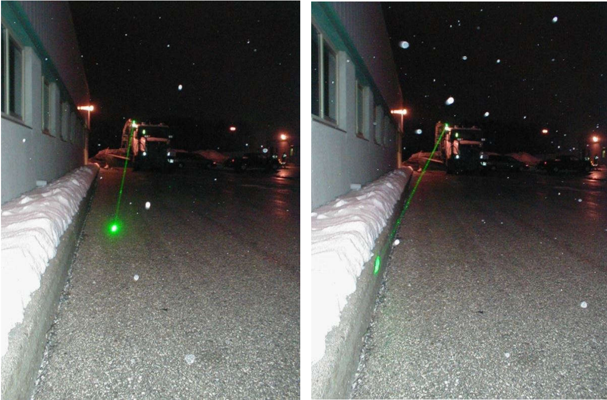
Figure 3-46 Laser projection in action showing outside edge of wing plow of a winter operations vehicle (Laserline, 2018)
