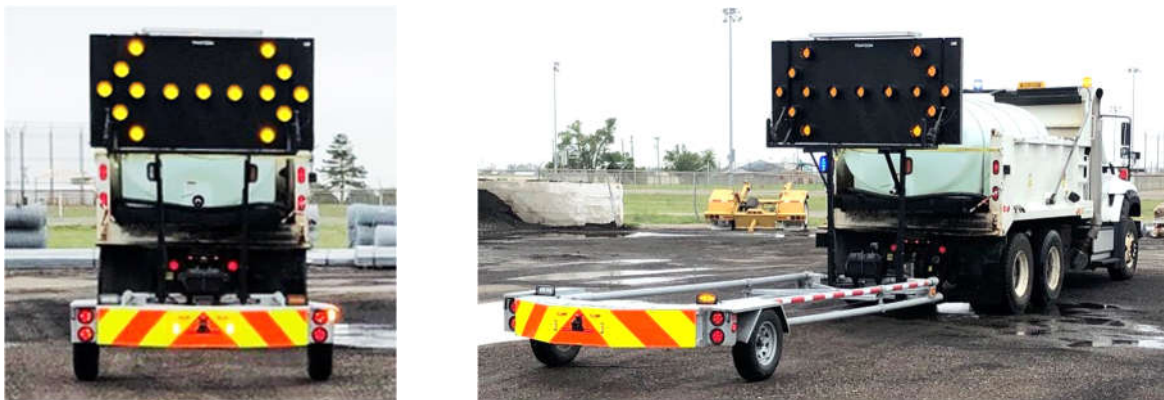
Figure 7-4 Recommended arrow board on the back of a winter operations vehicle (Shahandashti et al. 2019)
