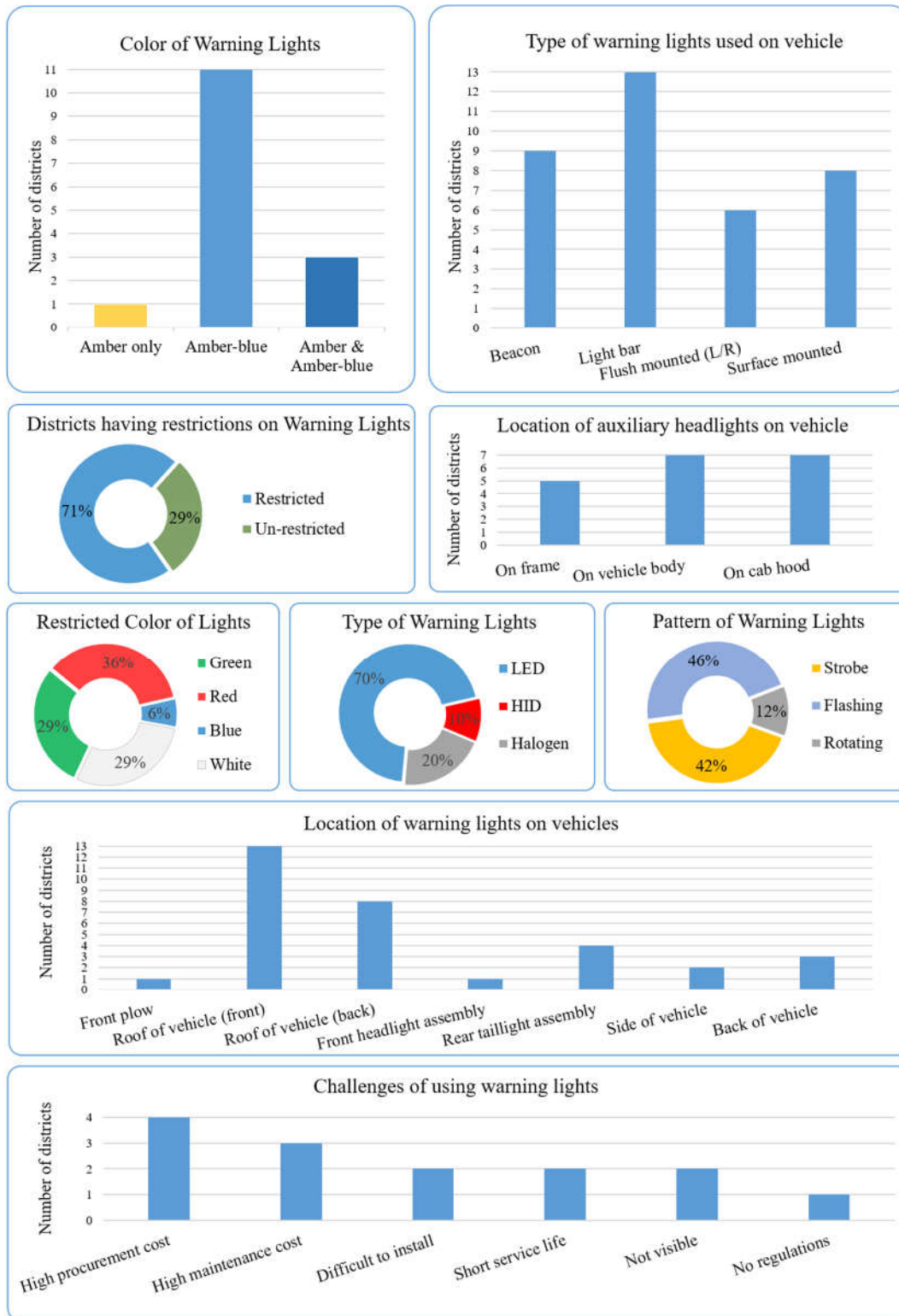
Figure 4-16 Survey results of 15 TxDOT districts on the evaluation of the warning lights on winter operations vehicles (Shahandashti et al., 2019)
