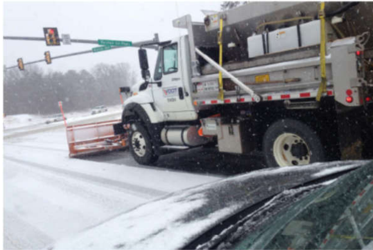
Figure 3-22 A winter operations vehicle of Virginia DOT with red and white retroreflective markings on the side (Washington Top News, 2015)
