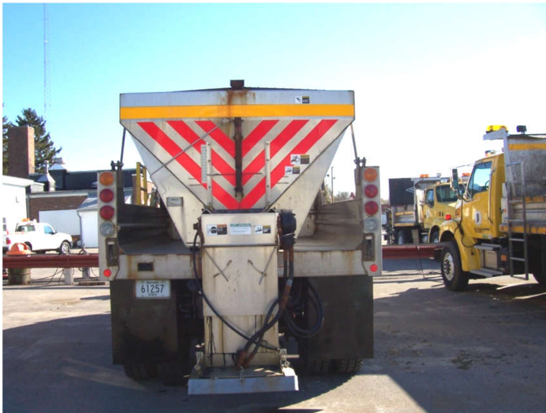
Figure 3-25 Warning sign on the back of Indiana DOT V-Box spreader (McCullouch and Stevens, 2008)
