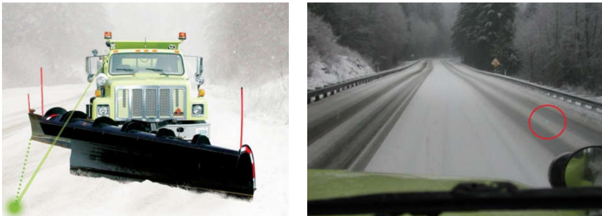
Figure 3-43 Laser path guidance system illustration and actual laser projection on the road from a winter operations vehicle (Laserline, 2018)
