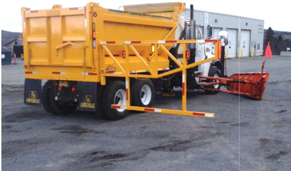
Figure 3-21 Safety Swing Arm with retroreflective markings (SNC Lavalin O&M, 2017)
