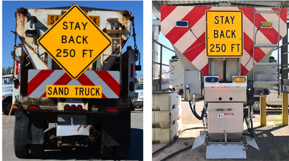
Figure 7-3 Recommended message signs on the back of winter operations vehicles (Shahandashti et al., 2019)
