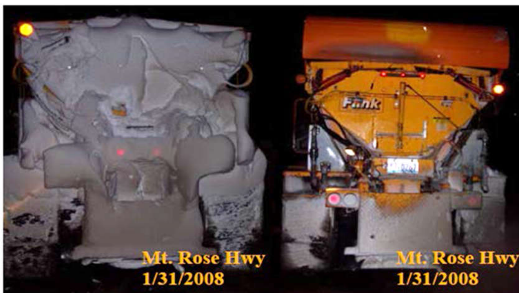
Figure 3-27 Airfoil test: Without airfoil and more snow accumulation on the rear (left) and with airfoil and less snow accumulation on the rear (right) (NDOT, 2008)
