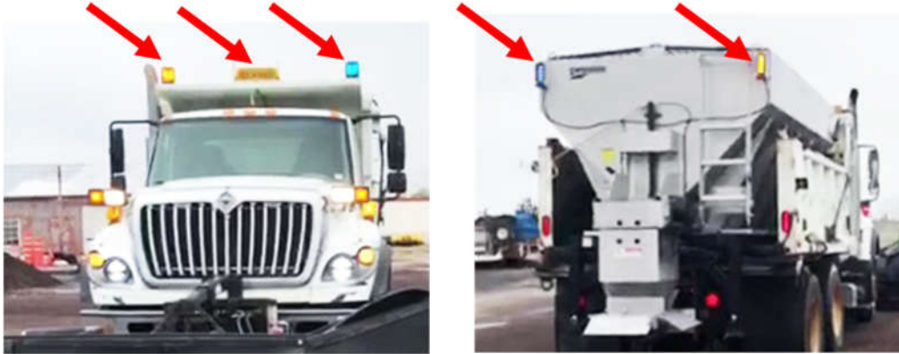
Figure 7-1 Recommended amber and blue color warning lights on top of winter operations vehicle (Shahandashti et al. 2019)
