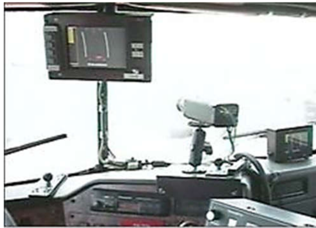
Figure 3-42 ASP Human-Machine Interface is mounted on the windshield of a Caltrans snowplow (FHWA, 2001)
