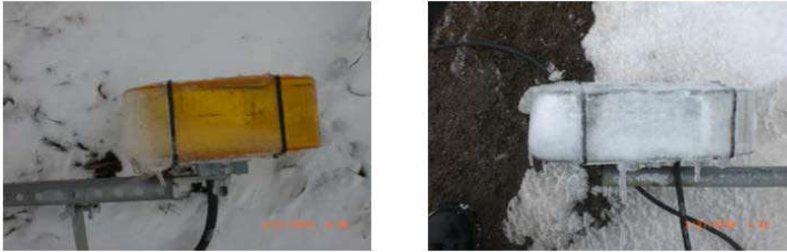
Figure 3-2 Comparison between HID (left) and LED (right) Lights after Heavy Snow Conditions (Vogt and Miller, 2008).
