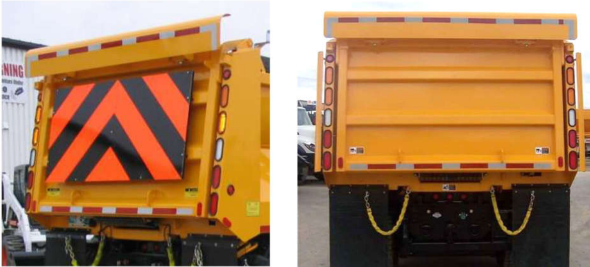
Figure 3-20 Red and white retroreflective tape fully outlining the rear tailgate of a winter operations vehicle in Ontario (Dow & Pearsall, 2014)
