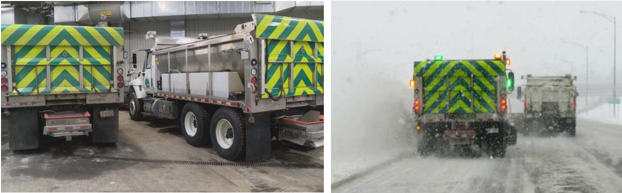
Figure 3-23 Warning signs on the back of winter operations vehicles in Ohio (ODOT, 2018 (left); Barbaccia, 2014 (right))
