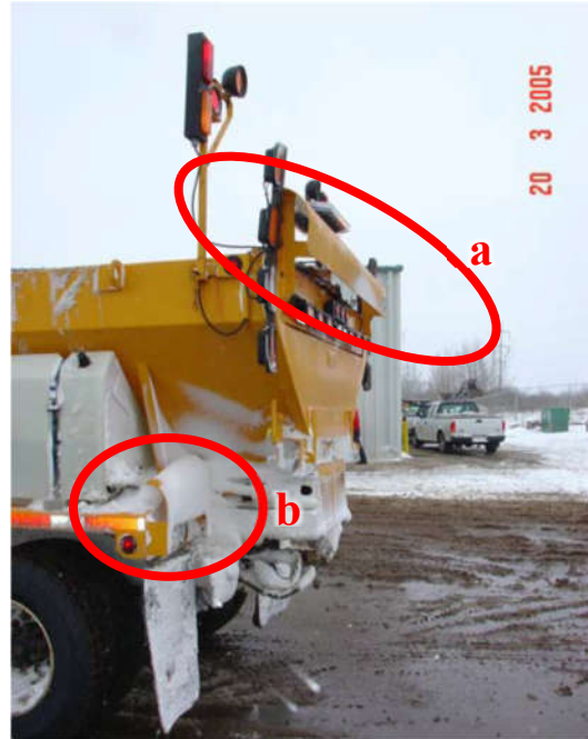
Figure 3-30 Side view of a winter operations vehicle showing: (a) Rear airfoil mounted on top of the vehicle and (b) Box wind deflector mounted on top of the taillight (Paulichuk, 2005)
