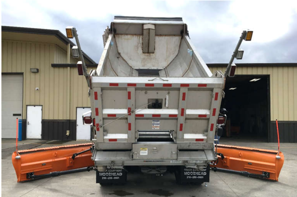
Figure 4-10 Back view showing wing plows of winter operations vehicles of North Dakota (Shahandashti et al., 2019)
