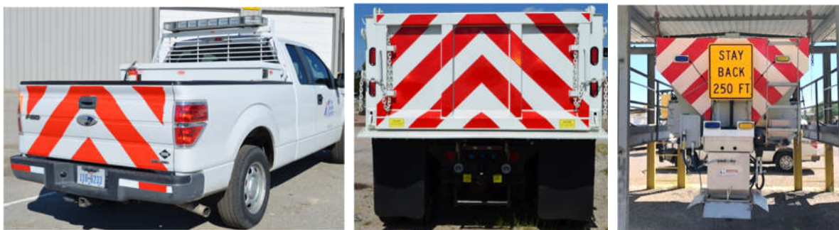
Figure 7-5 Recommended retroreflective markings on the back of winter operations vehicles (Paris (left), Wichita Falls (middle) and Dallas (right) Districts) (Shahandashti et al. 2019)
