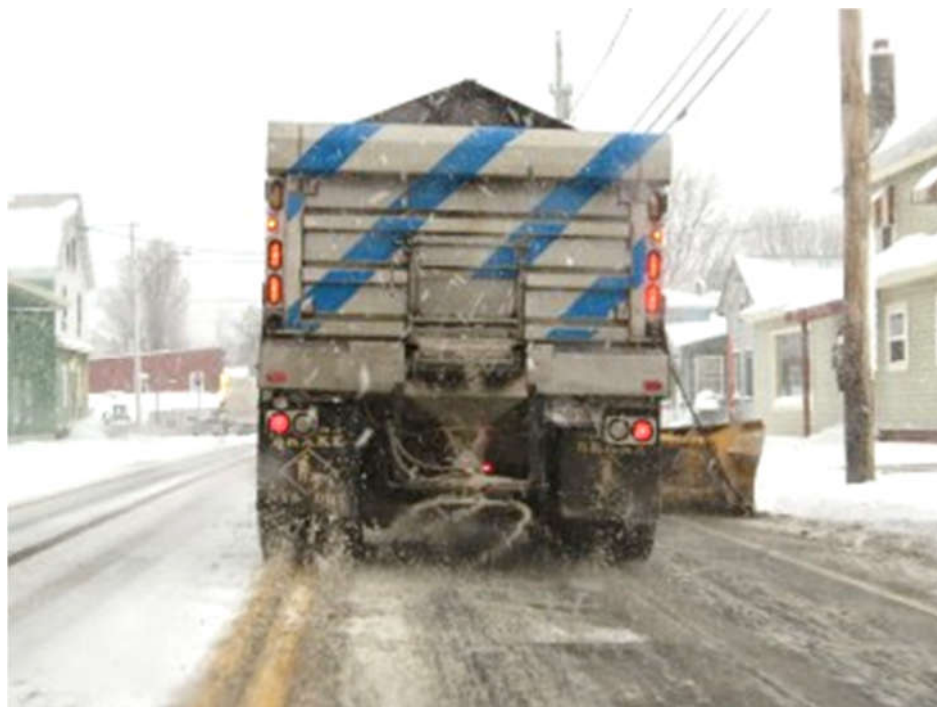
Figure 3-26 Warning signs on the back of a winter operations vehicle in Connecticut (CT Mirror, 2015)
