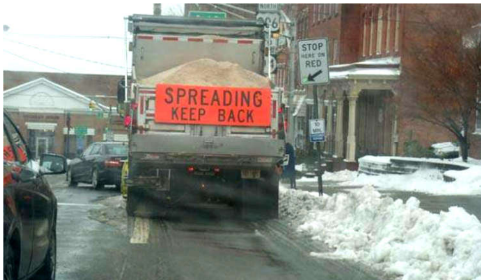
Figure 3-13 Message sign on the back of a winter operations vehicle of Sussex County, New Jersey (New Jersey Herald, 2012)
