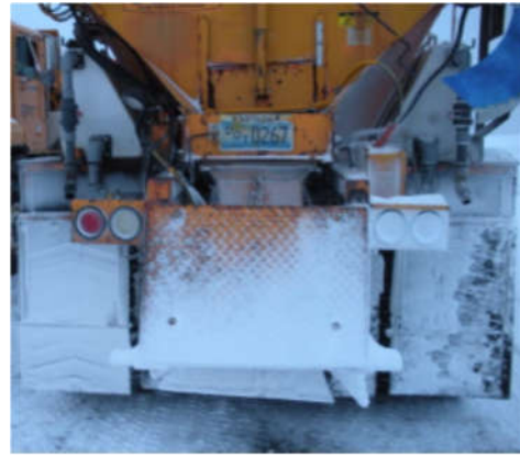
Figure 3-29 Side wind deflector on a winter operations vehicle (NDOT Class-15 Snowplow Truck) showing right taillight covered with snow despite the installation of the deflector (Dinc, 2011)
