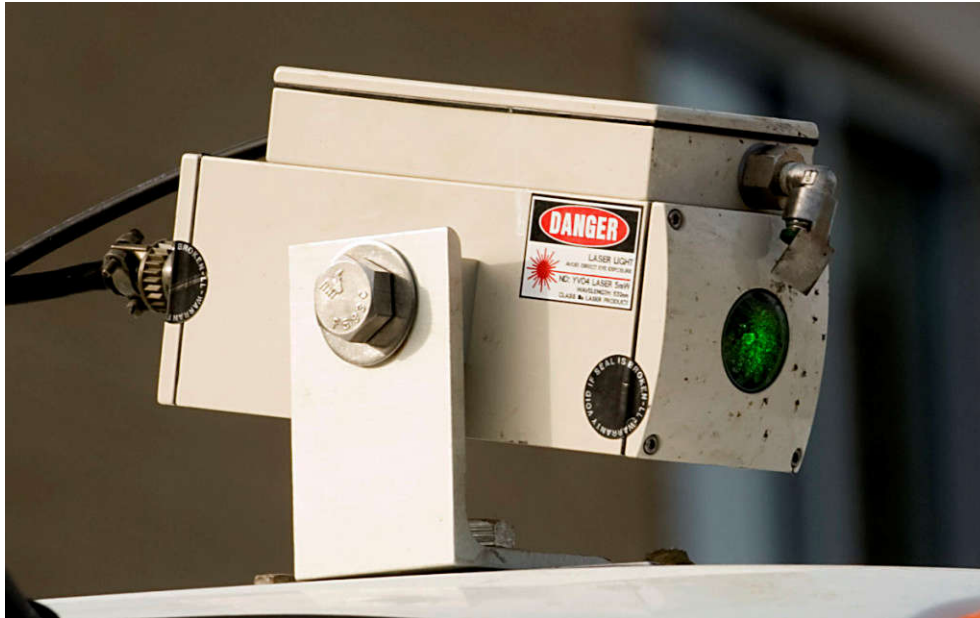
Figure 3-47 Bright green laser, as a guide to the trailing edges of snowplow trucks' wing plows, mounted on top of the trucks (Northern Virginia Daily, 2015)
