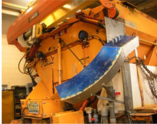
Figure 3-29 Side wind deflector on a winter operations vehicle (NDOT Class-15 Snowplow Truck) showing right taillight covered with snow despite the installation of the deflector (Dinc, 2011)
