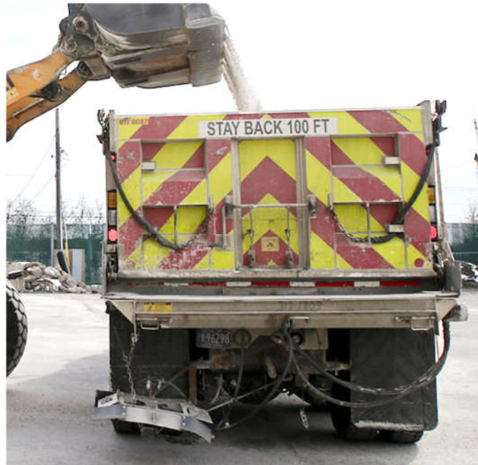
Figure 3-11 Message sign on the back of a winter operations vehicle in Pennsylvania (WITF, 2019)
