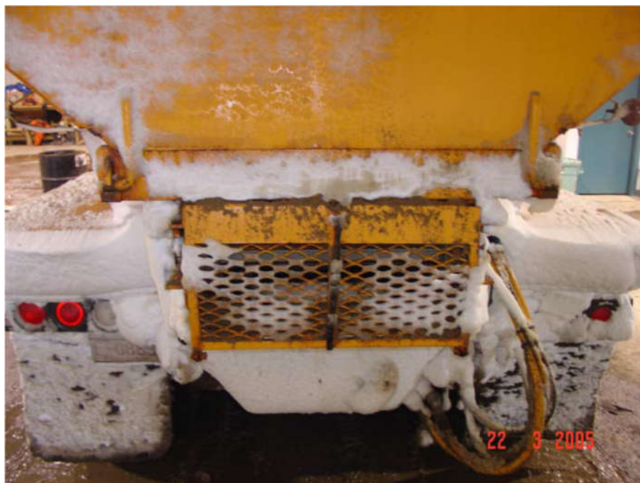
Figure 3-32 A direct comparison between the left and right taillights of a winter operations vehicle equipped with box wind deflectors. The right side is more heavily covered than the left side. (Paulichuk, 2005)
