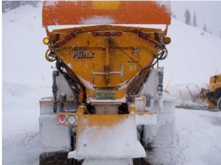
Figure 3-28 Airfoil keeping snow away from the back and left taillights of the winter operations vehicle but unable to keep snow away from right taillights. (NDOT, 2008)
