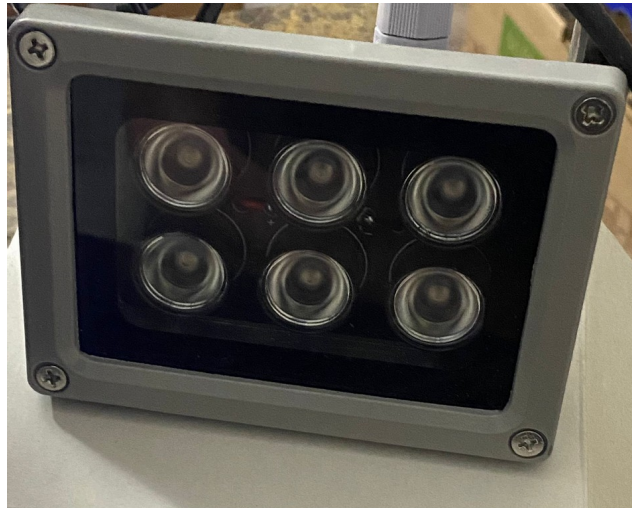
Figure 5: ES – IR1206U IR Illuminator
