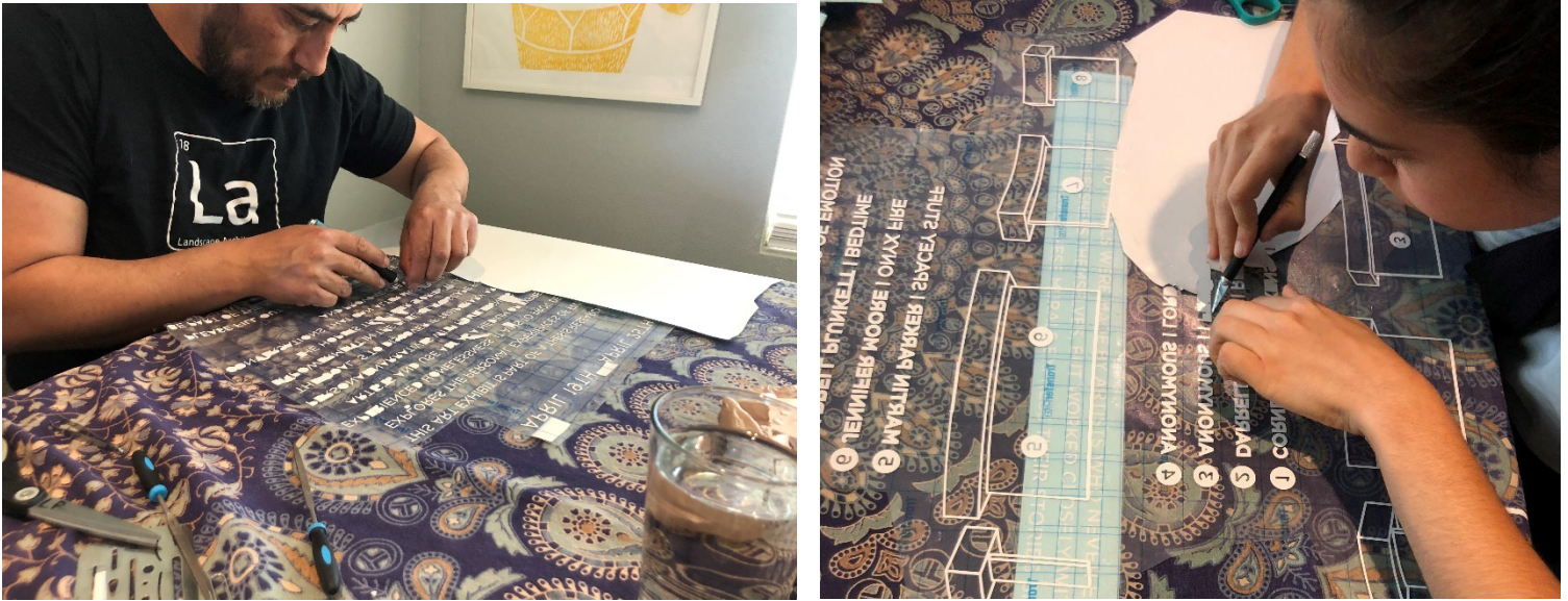
Figure 36 Signage Wall Vinyl Cut Weeding Process
