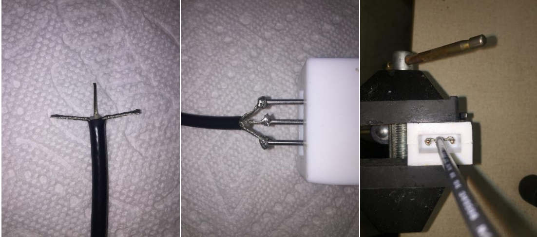
Figure 9. Fabrication process of the TDR sensors.
