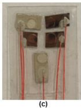
Figure 6- 1. (a) Graph of the sensor-array placed on the lamination pouch. (b) Graph of the end product of the sensor-array. (c) Photo of the sensor-array.
