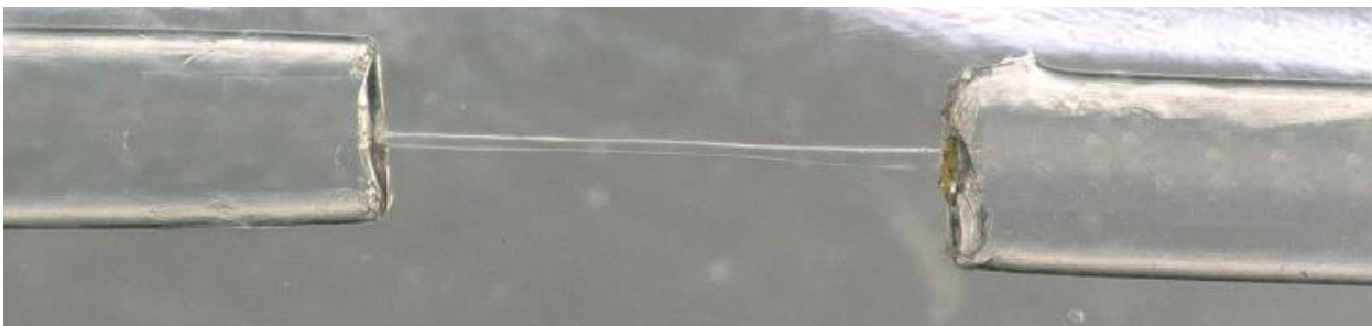
Figure 3-5 Prepolymer solution (PVA-SS25) cast microchannel , ca. 1500 \mu\text{m} long, 30 \mu\text{m} in diameter. The larger connecting channels, originating from 360 \mu\text{m} o.d. guide capillaries, are \sim 400 \mu\text{m} in i.d.
