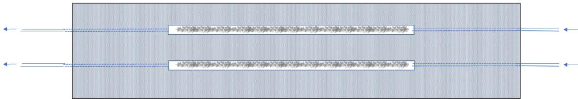
Figure 23: Two channel PDMS SERS device with silver dendrites
