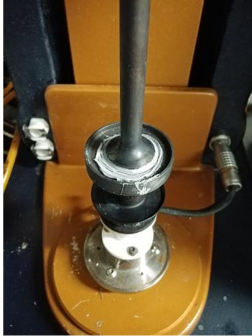
Fig. 62: Sample placed between two parallel plates of Discovery Hybrid Rheometer (HR-2).
