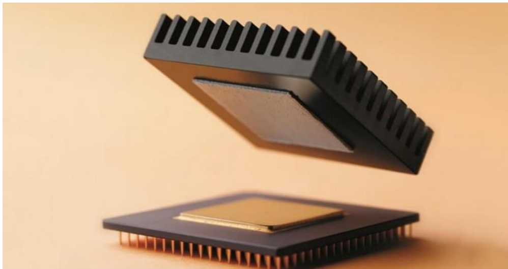
Fig. 56: Thermal Interface Materials [50].
