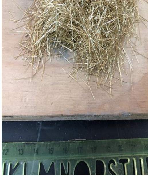
Figure 2: Actual steel fibers utilized in the experimental work
