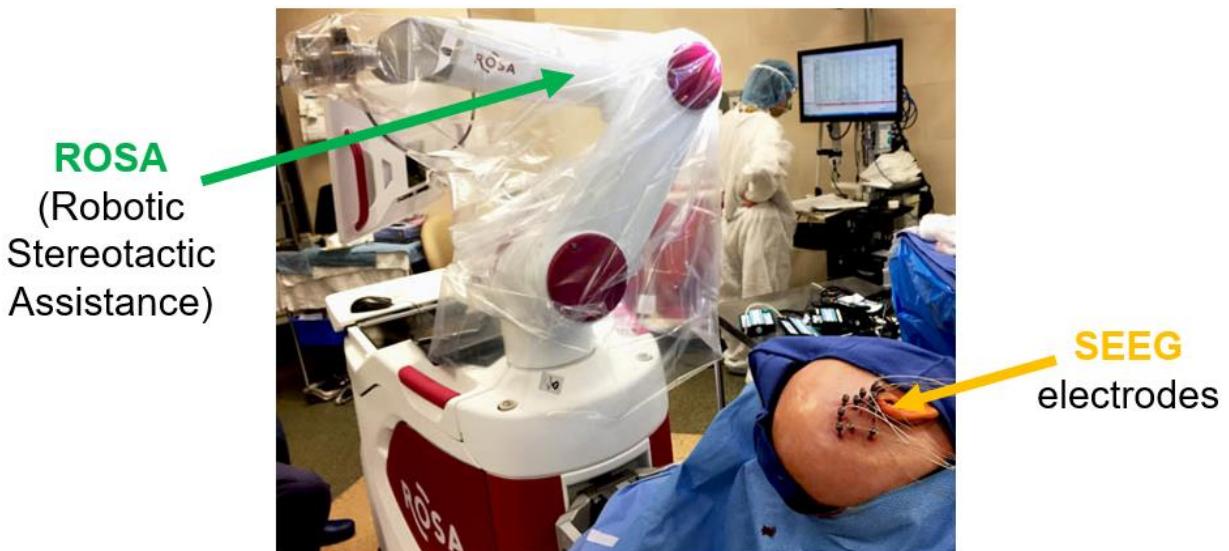
Figure 7. The Robotic-Guided Stereotactic EEG (ROSA) arm placed in the “home” setting after precise placement of SEEG electrodes [42].
