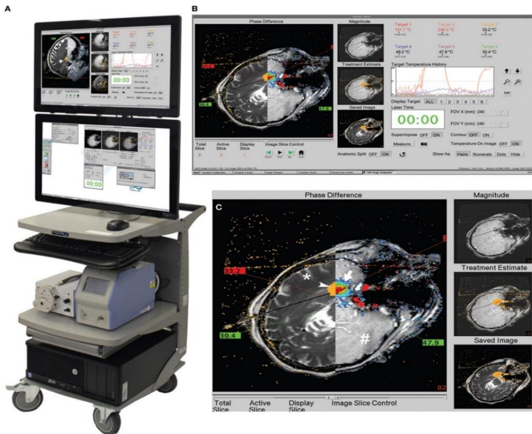
Figure 8. A) Visualase workstation without the arm, with two monitors, the peristaltic pump for the coolant on the bottom level of the station to the left, and the diode laser to the right to the right. B) A screen shot of the top monitor while the bottom monitor allows you to toggle between images and viewpoints, C) a closeup of the heat map in real time of the top monitor with the irreversible damage zone versus ablation zone [44].
