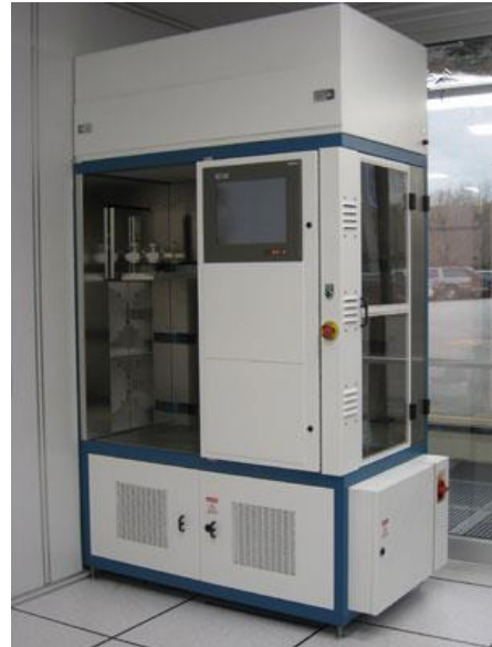
Fig. 3-2. LPCVD System for \text{Si}_3\text{N}_4 layer deposition located at UTA Cleanroom [62].
