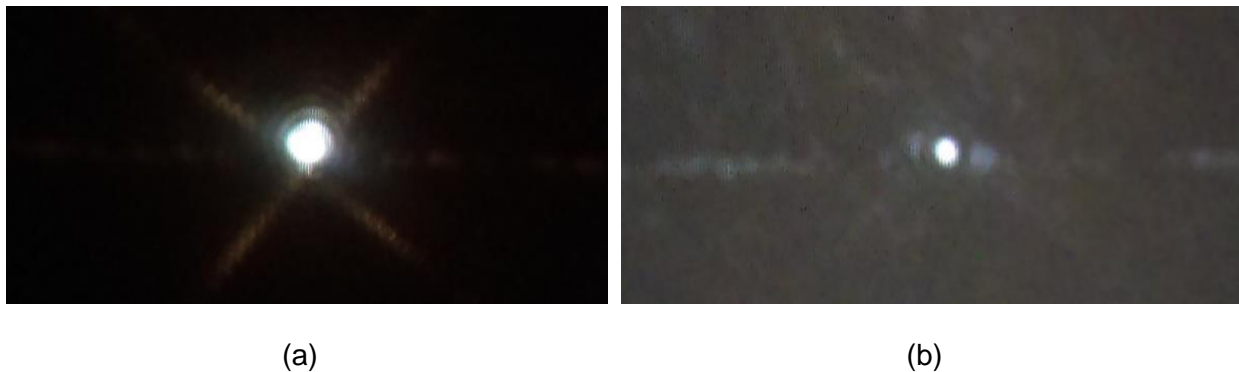
Fig. 3-10. Mode profile of (a) Visible light beam and (b) IR light beam at 1550 nm
