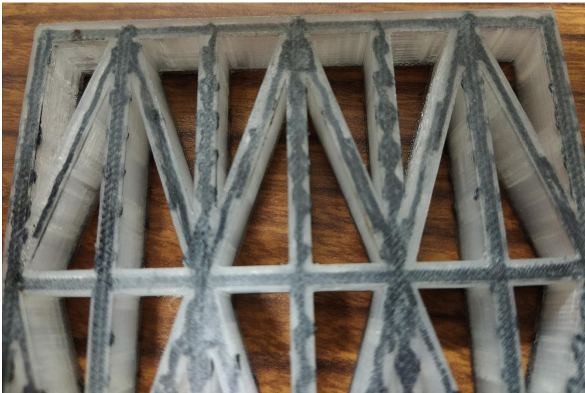
Figure 41 Fiber discontinuity and curling
