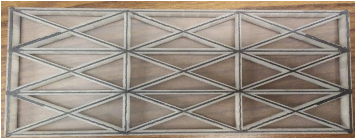
Figure 39 Grid angled grid superimposed on orthogrid
