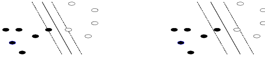
Figure 2.1. The decision line (solid) with the smaller and maximal margin. The data points on the dashed lines are the Support Vectors..
