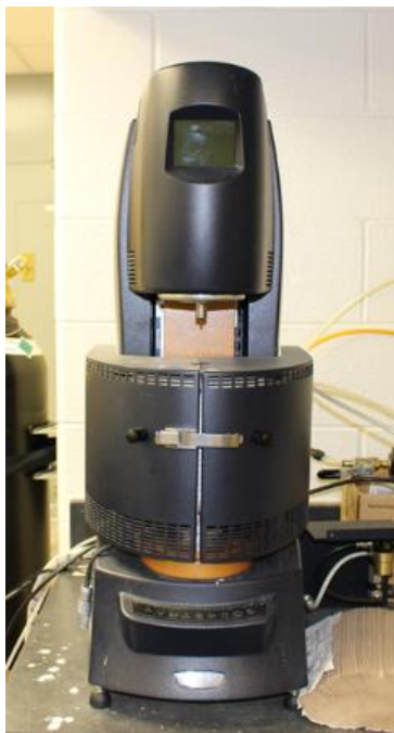
Figure 45 Discovery hybrid rheometer (HR-2, TA Instruments Inc.)
