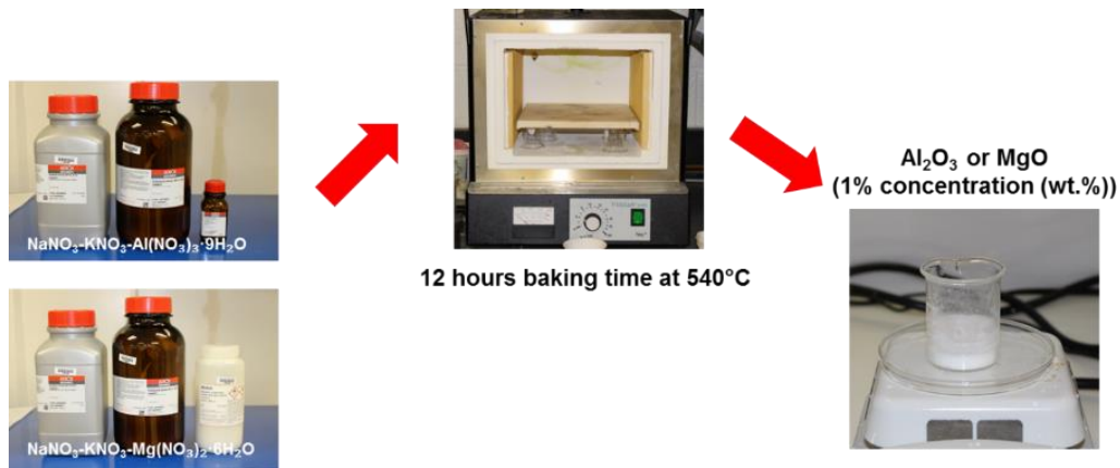
Figure 36 Procedure of the sample preparation of the nanofluid for the thermal decomposition process
