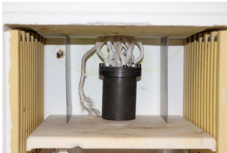
Figure 53 Customized cylinder in a laboratory furnace with two radiation shields
