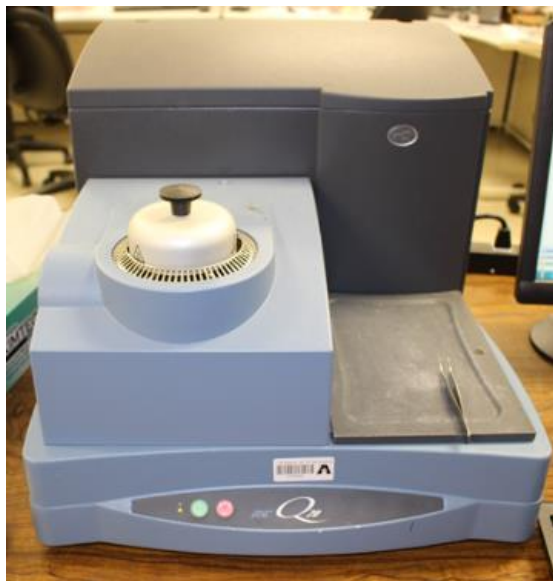
Figure 25 Modulated differential scanning calorimeter (MDSC; Q20, TA Instruments Inc.)
