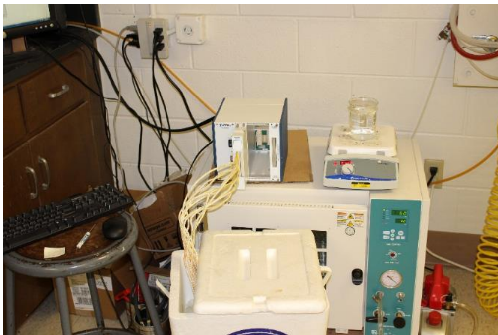
Figure 56 Set-up of the calibration of each thermocouple with DAQ system
