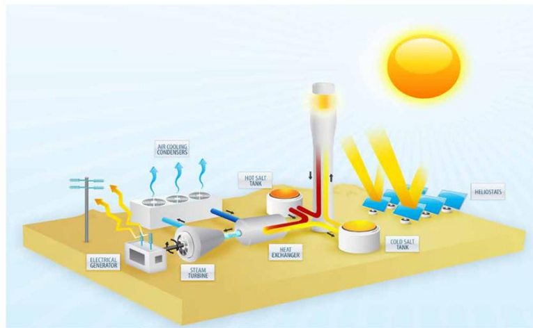
Figure 2 Schematic of the concentrated solar power (CSP) system [2]
