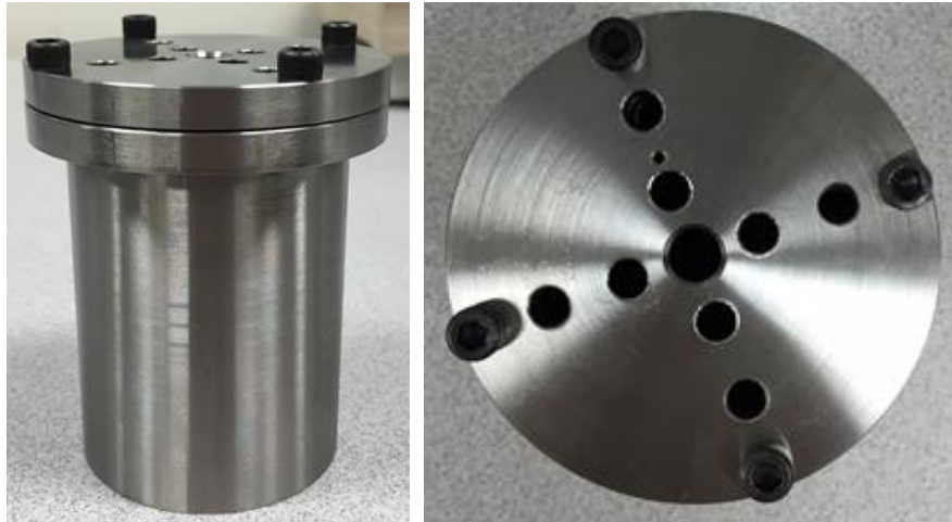
Figure 52 Customized cylinder includes four holes in the inner cylinder and four holes in the outer cylinder for the temperature measurement
