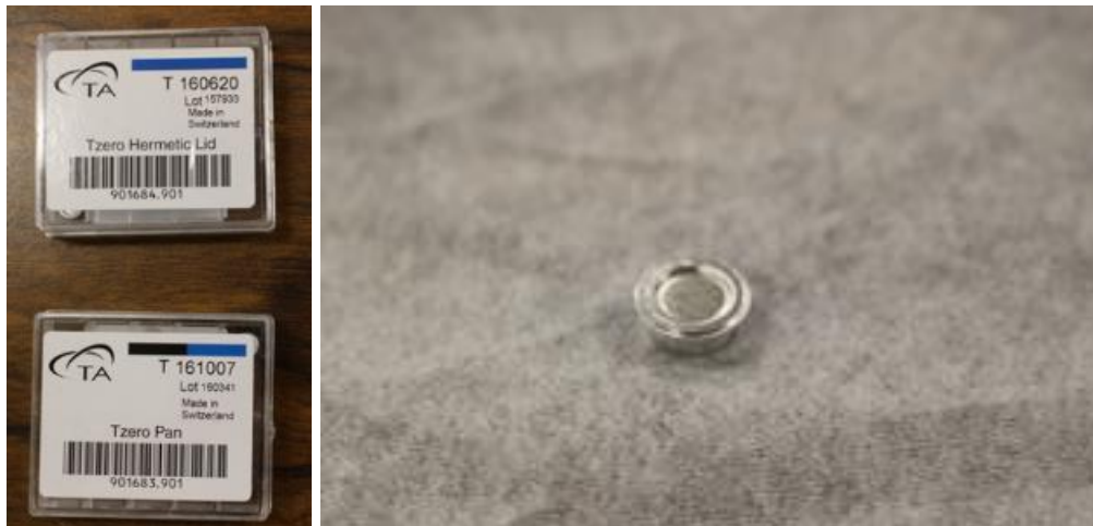
Figure 26 Tzero hermetic pan and lid (TA Instruments Inc.)
