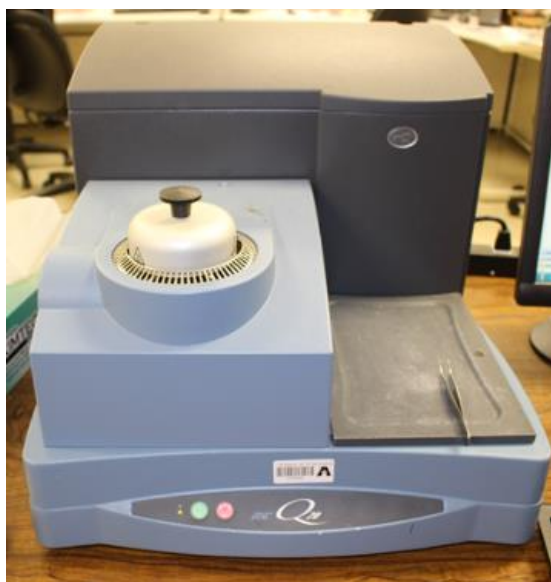
Figure 37 Modulated differential scanning calorimeter (MDSC; Q20, TA Instruments Inc.)
