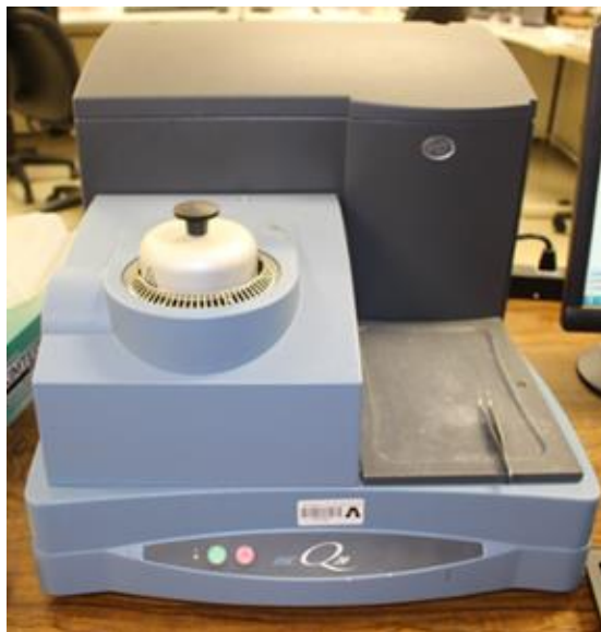
Figure 67 Modulated differential scanning calorimeter (MDSC; Q20, TA Instruments Inc.)
