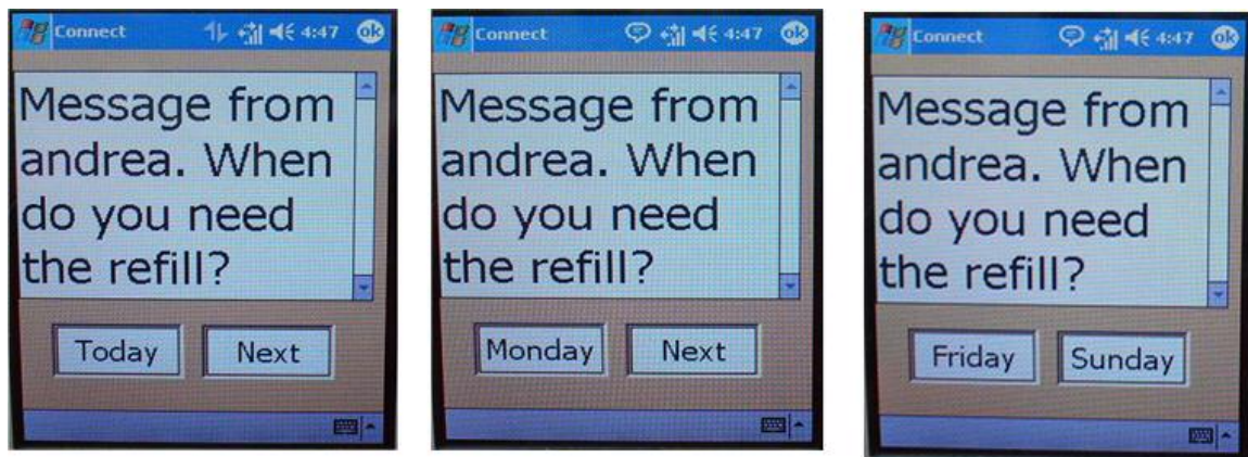
Figure 3.14. A four response choices message presented on a Pocket PC. The figure shows three touch screen supported Pocket PC interfaces for a message with four response choices. The first interface shows a reminder message displayed in a touch screen, which reads “Message from andrea. When do you need the refill?” and has two touch screen response choices, “Today” and “Next”. The second interface shows the same reminder message displayed in a touch screen and has two touch screen response choices, “Monday” and “Next”. The third interface shows the same reminder message displayed in a touch screen and has two touch screen response choices, “Friday” and “Sunday”. The titles of all screens are “Connect”.
