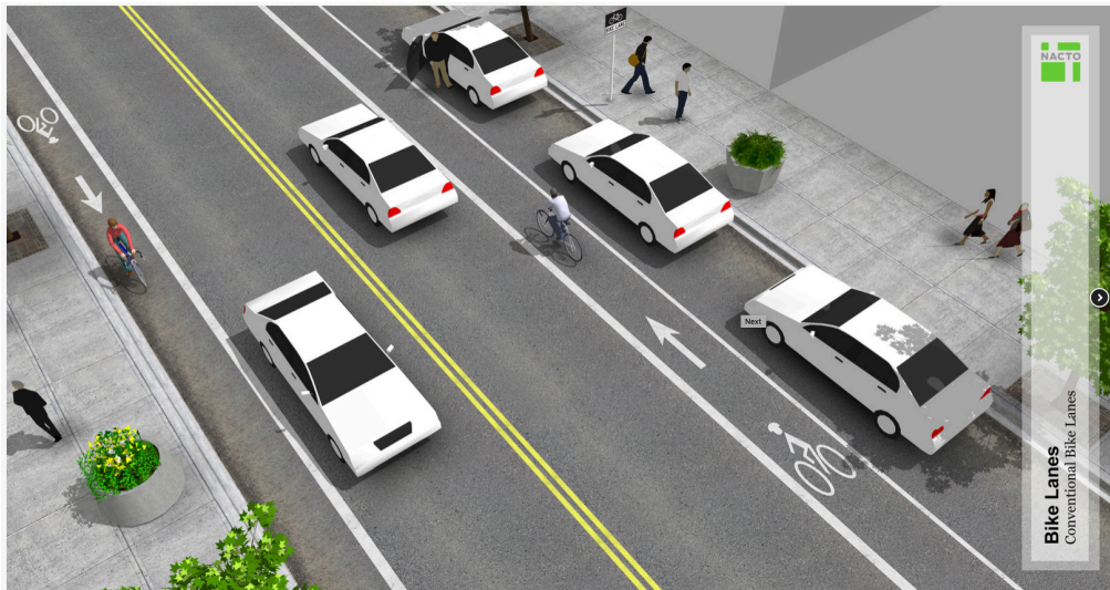
Figure 27: Narrowed main lanes creates space for parallel parking and bike lanes. Credit: NACTO.
