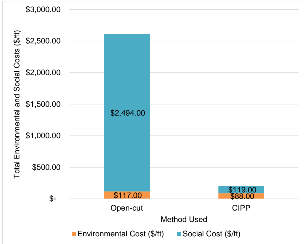
Figure 4-12 Total Environmental and Social Costs of CIPP Renewal and Open-cut Pipeline Replacement for Small Diameter Sanitary Sewers
