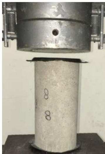
Figure 33. Compressive strength tests for an 8 PCY (0.52% V_f ) specimen
