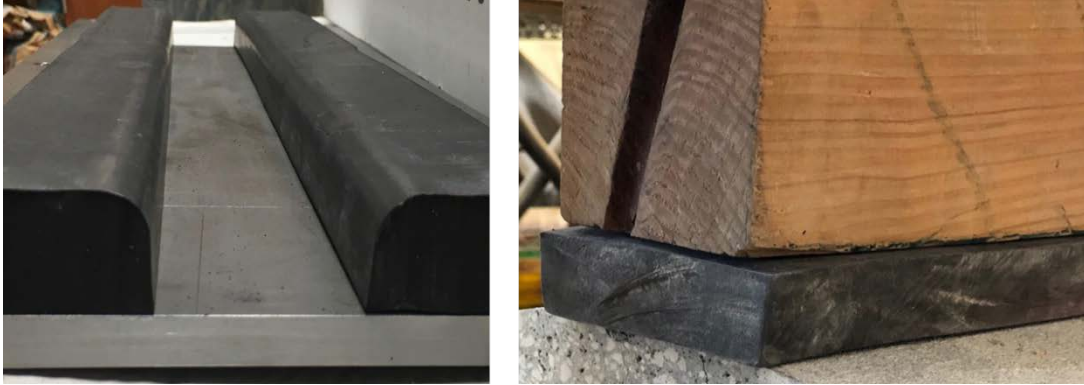
Figure 65. Rubber edges of the three-edge bearing tests
