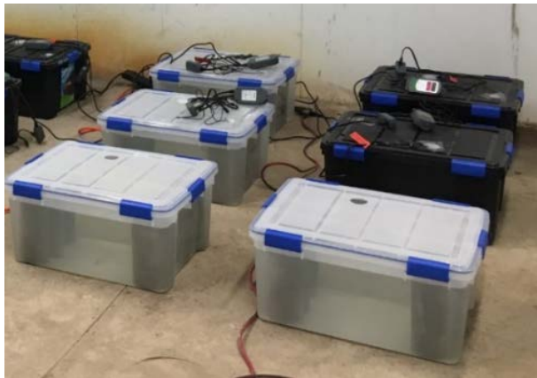
Figure 35. Cylinders aging in sulfuric acid and elevated temperature
