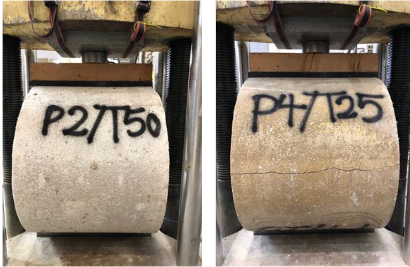
Figure 87. Three-edge bearing tests, one-year immersion
