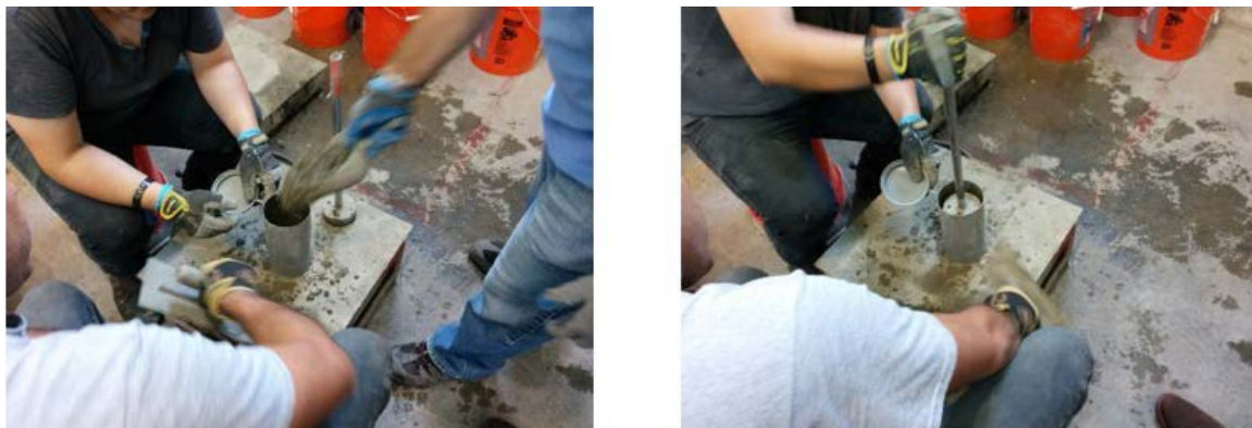
Figure 32. Specimen casting and compaction
