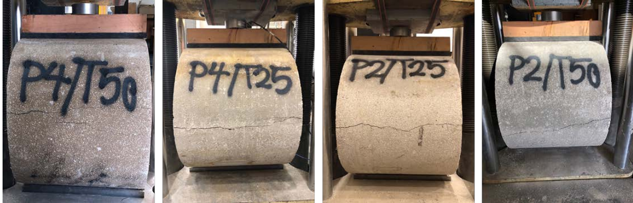
Figure 82. Three-edge bearing tests, five months of immersion
