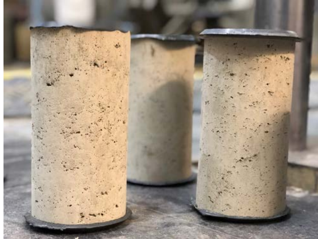
Figure 34. Sulfur capped specimens
