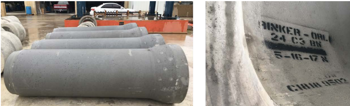
Figure 48- Twenty four-inch synthetic fiber reinforced concrete pipes
