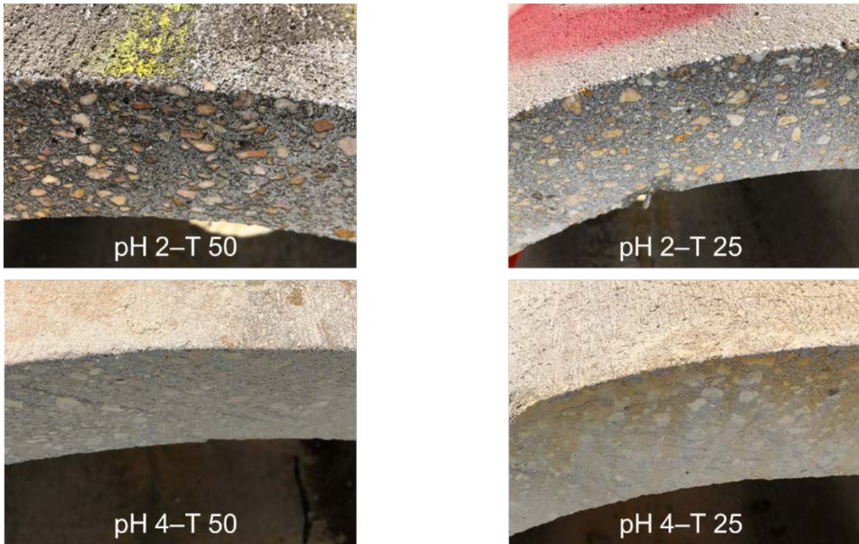
Figure 71. Post-immersion specimens' surface, 2 months tests
