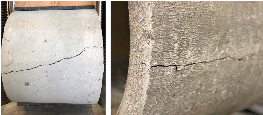
Figure 66. SYNFRCP at the ultimate load
