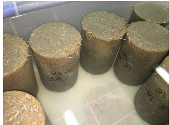
Figure 35. Cylinders aging in sulfuric acid and elevated temperature
