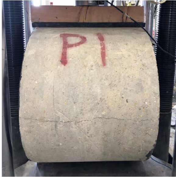
Figure 47. Three-edge bearing test
