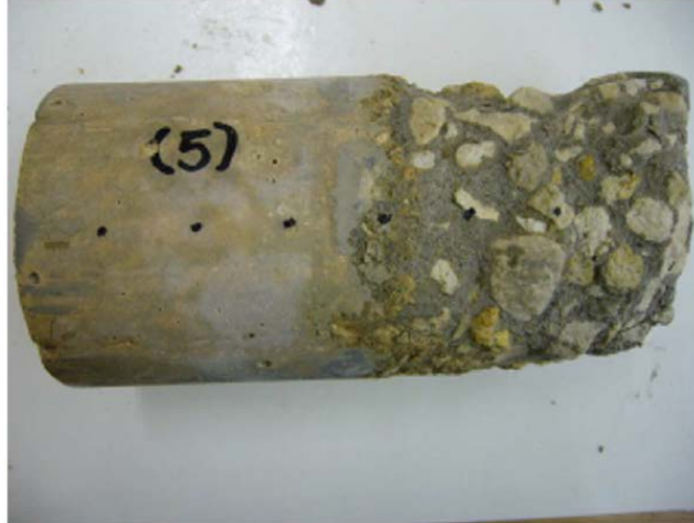
Figure 27. Sulfate attack on a concrete cylinder, Hartell and Boyd [32]
