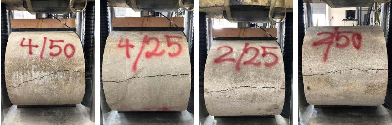
Figure 72. Three-edge bearing tests, two months immersion
