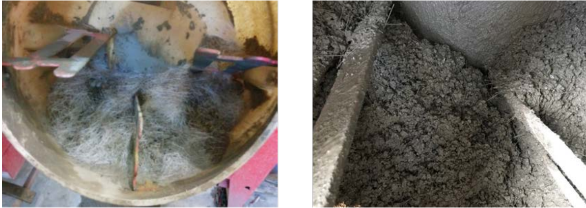
Figure 31. Uniform distribution of fibers and concrete mix
