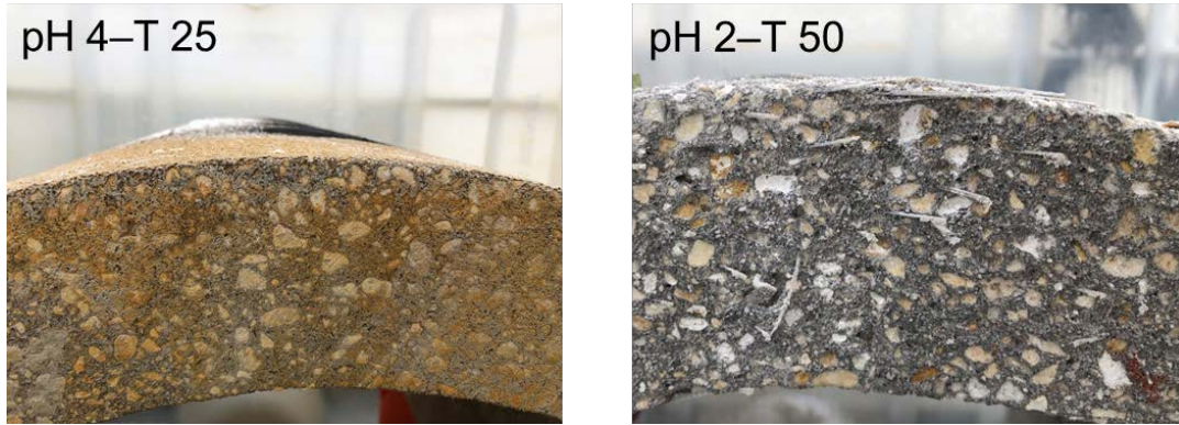
Figure 85. Post-immersion specimens' surface, 8 months tests
