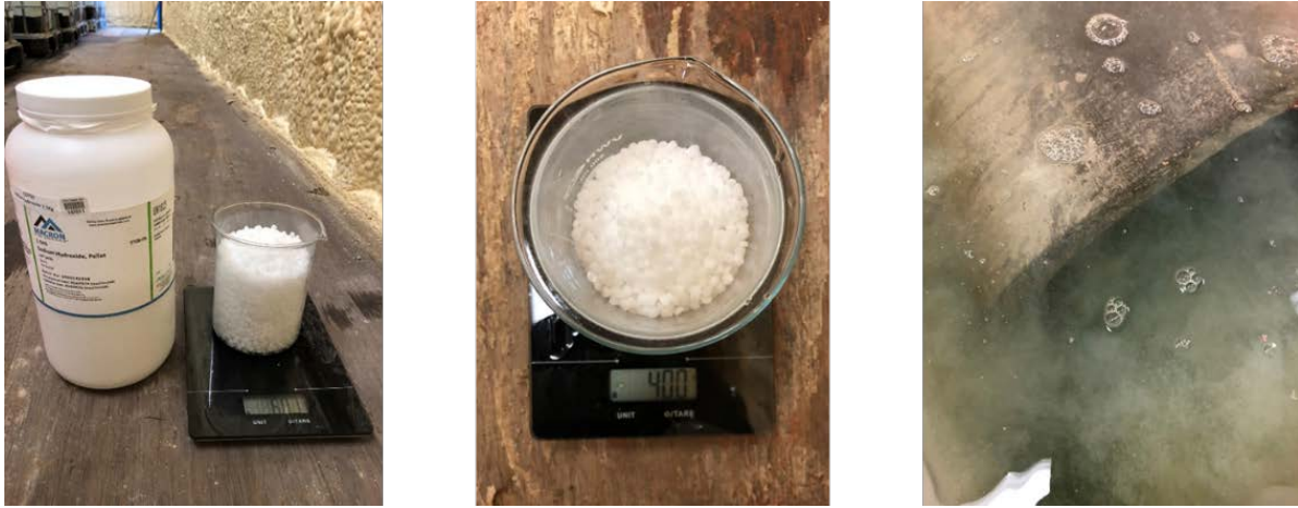
Figure 70. Sodium Hydroxide and acidic solution neutralization
