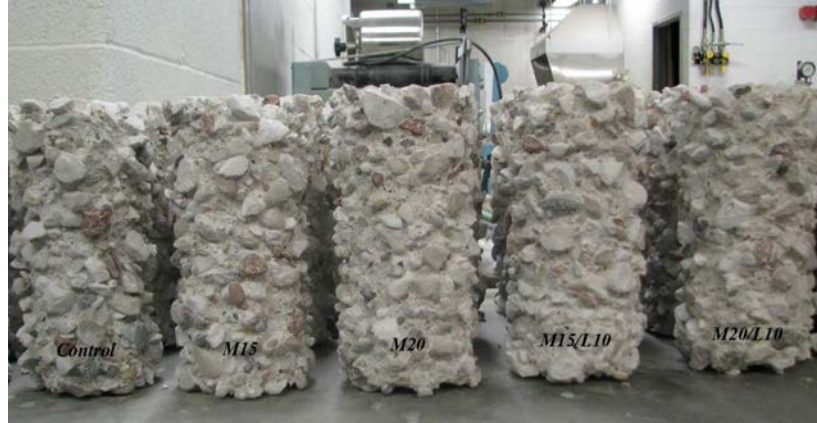
Figure 29. Visual assessment of degraded concrete samples after 8 weeks of exposure to a 5% sulfuric acid solution, Joorabchian [34]
