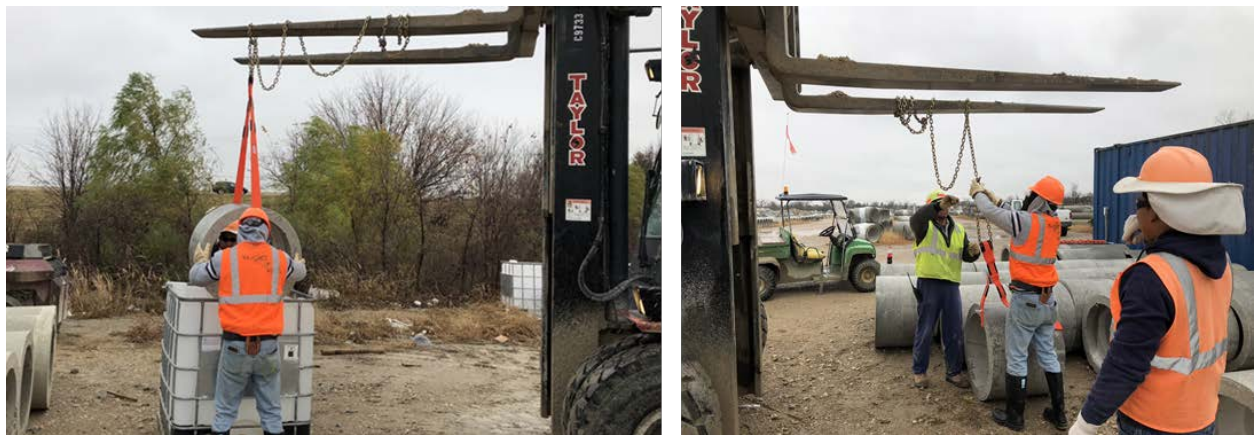
Figure 61. SYNFRCPs adjustment in 275-gallon totes
