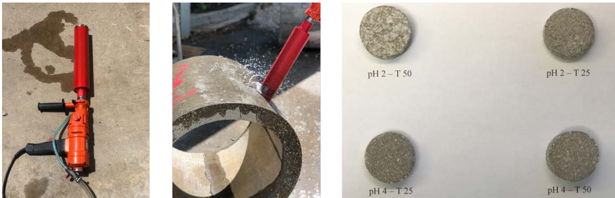
Figure 92. Coring and SEM sample preparation
