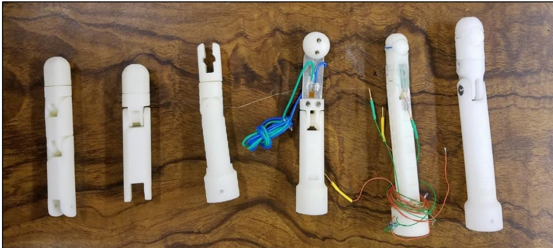
Figure 3.3 – Some the prototyped revisions of the Smart Finger (oldest to newest, left to right)
